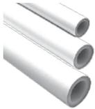
Diffusion-resistant PEX pipes, five-layer (PEX – adhesive agent – oxygen barrier – adhesive agent – PEX), for general plumbing and radiator connection applications. Manufactured to ISO 15875 for hot and cold water and heating applications with full WRAS approval.
