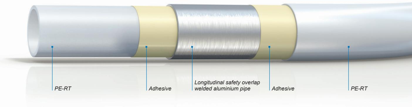
**The Uponor MLC pipe for tap water installation, radiator and fan-coil connection can also be ordered pre-insulated (up to 25 mm). You have an assortment available in sizes from 16 – 110 mm. The pre-insulated pipes save installation time because the time intensive insulation of the mounted pipes and the resulting gluing of joints are eliminated.**
