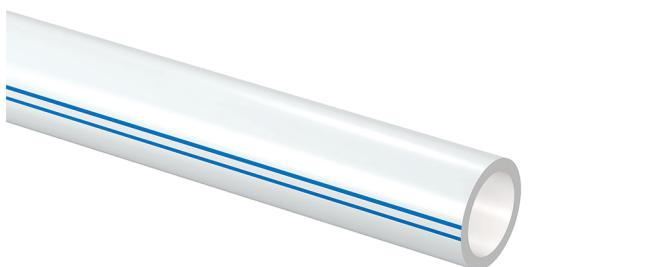
Uponor Comfort Pipe PLUS is a highly flexible PE-Xa pipe with 5 layers available in the dimensions 14 x 2,0 mm, 16 x 2,0 mm and 17 x 2,0 mm.
