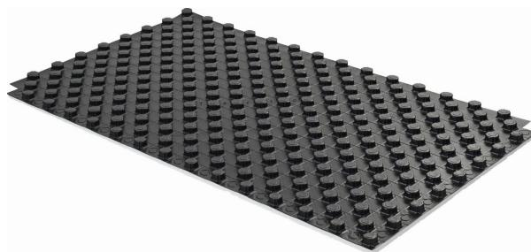
The Uponor Tecto nub panel ND 11 is a back-foamed EPS insulation panel, available with two-sided overlapping foil for a screed-tight connection and is suitable for 14 mm - 17 mm pipe dimensions.
