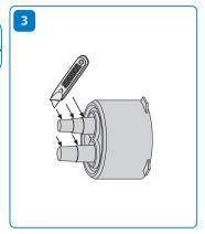
Open outlets on the rubber end cap according to the flow pipe size.
