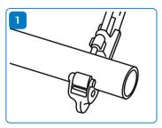
Cut the pipe at a right angle using a pipe cutter intended for plastic pipes.
