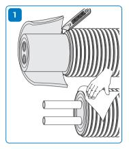
Cut away jacket pipe and peel off insulation layers so that enough flow pipe is visible to join the coupling and the end cap. Be careful not to damage the flow pipe. Clean the surfaces carefully.
