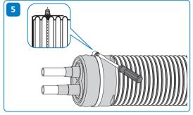
Position the jubilee clip over the seal and tighten.
