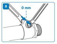
Tighten the outer sleeve so that its jaws touch. Tighten again carefully. If the jaws do not touch, wait for at least 30 minutes before re-tightening them.
