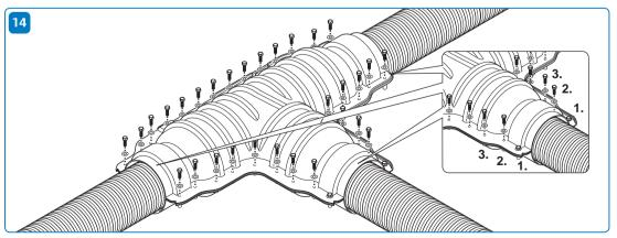
$\label{lem:complete} \textbf{Complete assembly of insulation set using bolts provided.}$
