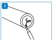
Bevel the pine from the inside using a bevelling tool or a knife and remove possible bevels left outside the pipe.
