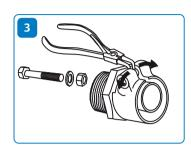
Remove the outer sleeve from the connector. Remove the bolt and spread the outer sleeve using a pair of pliers.
