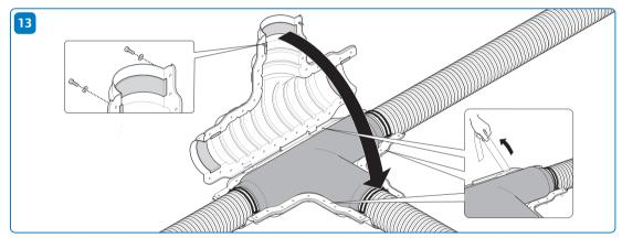
Fully release adhesive strips and position top half of casing over joint area.
