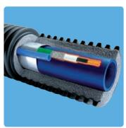
For liquids and water transport at extremely low temperatures, Uponor Supra Plus is supplied with a self-regulating freeze protection cable. It makes good sense to use this product if the pipeline is installed in conditions lacking weather protection, i.e. above ground or in shallow burial situations. The cable, rated at 10 w/m will prevent freezing down to -20°C.
