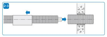
Install the shrink sleeve on top of the pipe element.
