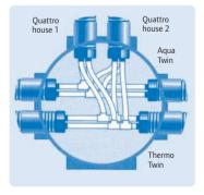
Heating and tap water from the main line to 2 houses using  $\mbox{\it Quattro}$
