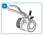
Place the bolt between the outer sleeve jaws and remove the outer sleeve.
