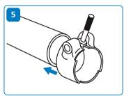
Push the outer sleeve over the pipe. Please note! Check that the outer sleeve has been turned in the correct position (the juts must be pointing towards the support sleeve). Installation of the pipe is easy and the o-ring remains undamaged when the o-ring is lubricated using a suitable lubricant (for example silicone spray).
