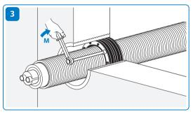
During final assembly, successively tighten up each nut with torque-wrench clockwise until the maximum torque Mmax is reached. Tighten the nuts several times. Repeate the procedure after two hours.
