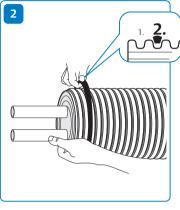
Install the rubber seal in the second groove.
