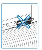
Insert the PWP wall seal as far as the water side (outside) – nuts face the cellar side
