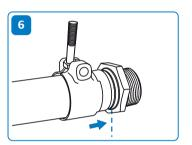
The pipe is pushed into the support sleeve all the way until the pipe stopper. Install the outer sleeve so that the anchoring groove is placed in the outer sleeve juts.
