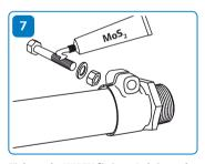
Tighten the WIPEX fittings. Lubricate the threads and washer of the bolt prior to tightening it. Use a suitable type of grease, such as silicone grease. Tighten the nut carefully using a spanner. Hold the bolt in place using a second spanner while tightening the bolt.
