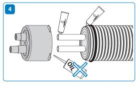
Install the end cap over the end of the pipe using lubricant. A non oil-based lubricant can assist.
