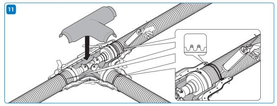
Position upper foam half-shell over joint area. Apply sealant to two corrugations where pipe meets spacer piece.
