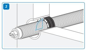
Install Uponor PWP wall seal pipe at right angles to Uponor pipe
