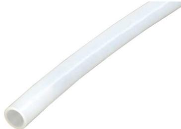
Note: Temperature and pressure ratings stated are hydrostatic ratings. For domestic hot-water (DHW) and DHW recirculation installations, operating conditions should not exceed 140°F (60°C) at 80 psi (5.5 bar) in accordance with ASTM F2023. For additional information regarding application-specific temperature and pressure ratings, refer to the Uponor PEX Piping Systems Design and Installation Manual.
