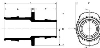
Note: Temperature and pressure ratings stated are hydrostatic ratings. For domestic hot-water (DHW) and DHW recirculation installations, operating conditions should not exceed 140°F (60°C) at 80 psi (5.5 bar) in accordance with ASTM F2023. For additional information regarding application-specific temperature and pressure ratings, refer to the Uponor PEX Piping Systems Design and Installation Manual.
