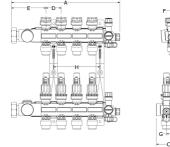
The Engineered Polymer (EP) Heating Manifold Assemblies feature isolation valves and balancing valves with flow meters (0-1 gpm), and come fully assembled, ready for installation in hydronic radiant heating and cooling systems. Use only propylene glycol in radiant systems with EP Heating the feature should be a shoul
