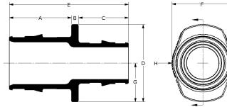
Note: Temperature and pressure ratings stated are hydrostatic ratings. For domestic hot-water (DHW) and DHW recirculation installations, operating conditions should not exceed 140°F (60°C) at 80 psi (5.5 bar) in accordance with ASTM F2023. For additional information regarding application-specific temperature and pressure ratings, refer to the Uponor PEX Piping Systems Design and Installation Manual.
