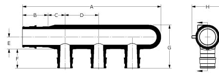
Note: Temperature and pressure ratings stated are hydrostatic ratings. For domestic hot-water (DHW) and DHW recirculation installations, operating conditions should not exceed 140°F (60°C) at 80 psi (5.5 bar) in accordance with ASTM F2023. For additional information regarding application-specific temperature and pressure ratings, refer to the Uponor PEX Piping Systems Design and Installation Manual.
