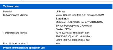
Use Uponor ProPEX® lead-free (LF) brass water meter service valves in all commercial submetering and residential water service inlets, outlets or both. The valves allow for a direct ASTM F1960 connection to water meters sized  $^5\!8"$  to 1". Valve is sized for  $^3\!4"$  or 1" Uponor AquaPEX® tubing. Product handle material is stainless steel.
