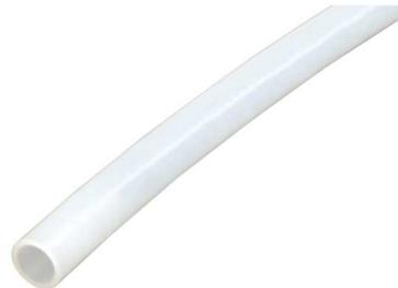
Note: Temperature and pressure ratings stated are hydrostatic ratings. For domestic hot-water (DHW) and DHW recirculation installations, operating conditions should not exceed 140°F (60°C) at 80 psi (5.5 bar) in accordance with ASTM F2023. For additional information regarding application-specific temperature and pressure ratings, refer to the Uponor PEX Piping Systems Design and Installation Manual.
