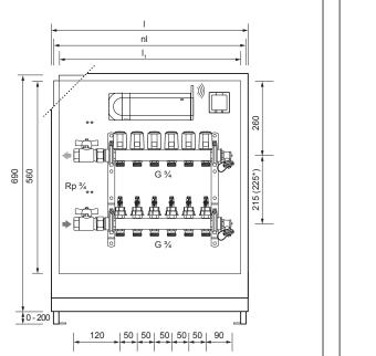
\* Vario M Manifold \*\* Optional: balancing valves or diff. pressure control valve
