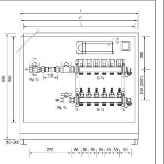
\* Vario M Manifold \*\* Optional: balancing valve or diff. pressure control valve
