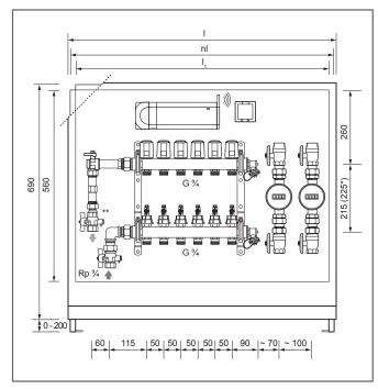
\* Vario M Manifold \*\* Optional: balancing valve or diff. pressure control valve
