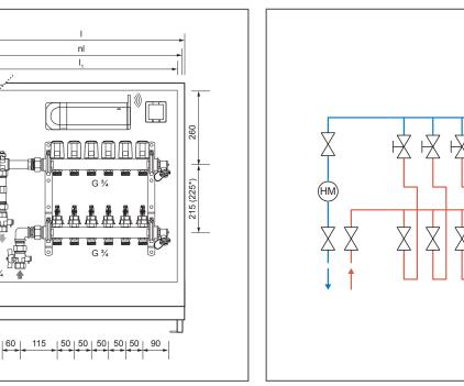
\* Vario M Manifold \*\* Optional: balancing valve or diff. pressure control valve
