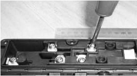
**Figure 3-23: Tighten screws**
