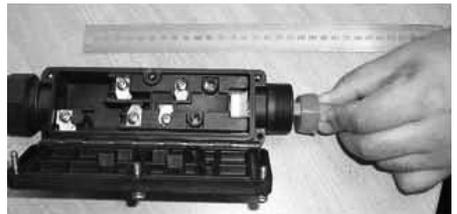
**Figure 3-21: Fasten seal and nut**
