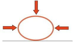
Weholite is subjected to external pressure. Weholite is a flexible pipe that absorbs external loads and deforms, which means that it will not crack.
