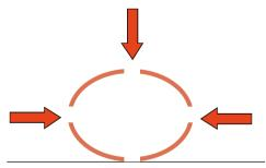
A rigid pipe is subjected to external pressure. The pipe does not deflect, and in the end it will crack.
