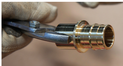
Figure 3-26 : Retirer le tuyau
