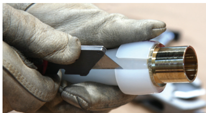
Figure 3-23 : Retirer la bague
