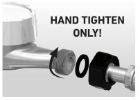
Step 3: Hand tighten assembly to meter. Add ½ turn, if needed. Note that overtightening may lead to potential leaks.
