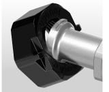
**Step 2:** Insert large tab into nut.
