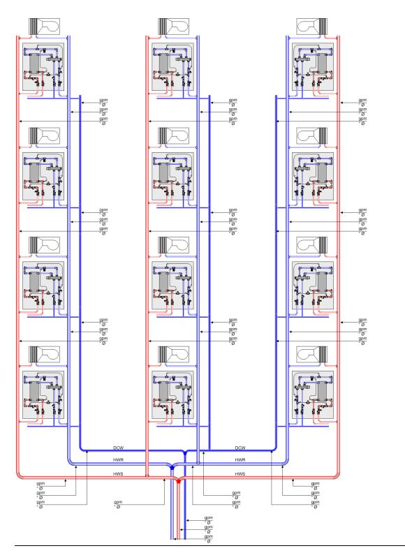
Figure 21: Example of a riser piping layout and dimensioning requirements for an AquaPort system. Note: It is advised that HTUs (i.e., fan coils, radiant floors, radiators, etc.) have return-temperature limiters to prevent unnecessary temperature increases through the heating plant.
