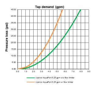
Figure 16: Pressure drop through HX = B16DW 40, on tap water side (secondary) for 5.25 U.S. gpm (19 L/min) warm-water tapping
