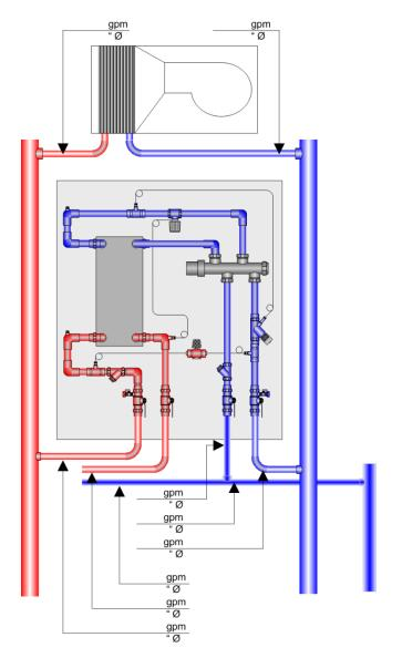
Figure 20: Dimensioning requirements for an AquaPort substation and HTU; includes flow, diameter, velocity, and differential pressure requirements
