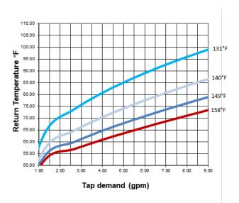
Figure 18: Hydronic return temperatures for HX = B16DW 40 when heating domestic water from 50°F ( $10^{\circ}$ C) to  $120^{\circ}$ F ( $49^{\circ}$ C)
