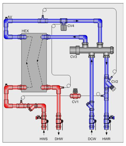
Figure 2: Standardized, factory-assembled substations for domestic hot water generation
