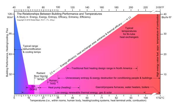
Figure 9: The relationship between building performance (y-axis), heat-exchanger sizing, and temperatures (x-axis). In essence, the larger the heat exchanger surface area to serve lower-flux results in a lower-temperature requirement more aligned with renewable systems, a fundamental principle in sustainability.
