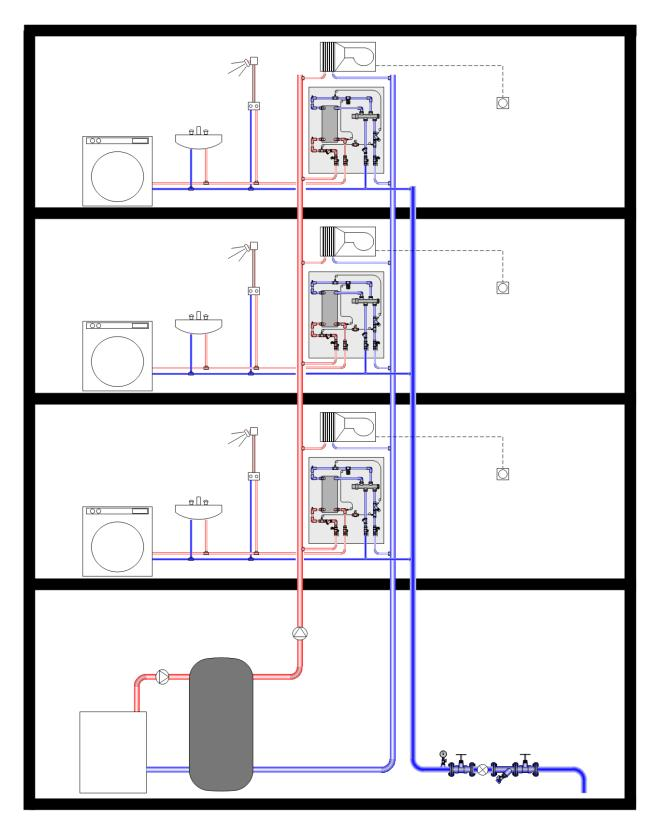
Figure 4: Application illustration for AquaPort substations in vertical-based district systems
