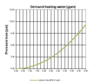
Figure 11: Pressure drop through HX = B16DW 20, on hydronic side (primary) for 3 U.S. gpm (680 L/h) warm water tapping
