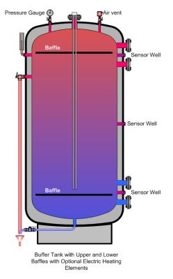
Figure 25: Highly insulated multiport buffer tank with baffles for promoting stratification
