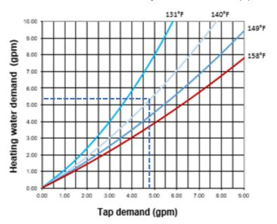
Figure 29: Performance curve for AquaPort 5.25 U.S. gpm
