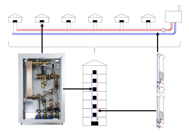
Figure 1: Typical district energy characteristics with heat-transfer stations (top illustration) rearranged into a vertical format (bottom illustration)
