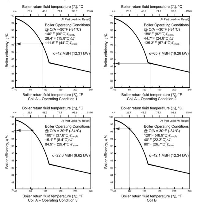
Figure 8: The effects of return water temperatures (x-axis) from heat exchanger selection on boiler efficiency (y-axis).
