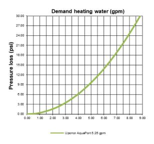
Figure 15: Pressure drop through HX = B16DW 40, on hydronic side (primary) for 5.25 U.S. gpm (1136 L/h) warm-water tapping
