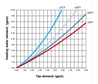
Figure 17: Supply temperatures and flow rates required for HX = B16DW 40 when heating domestic water from 50°F (10°C) to 120°F (49°C)
