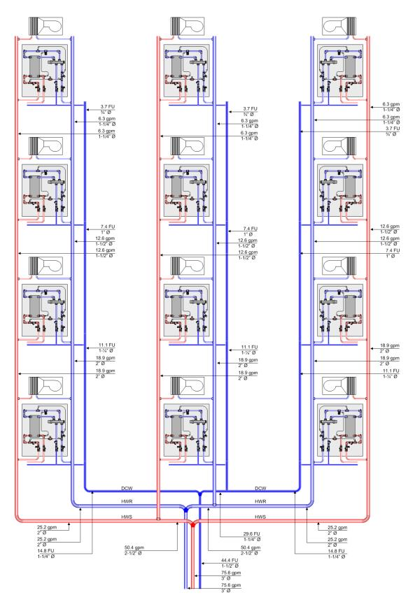
Figure 29: Riser diagram and dimensioning for the example given
