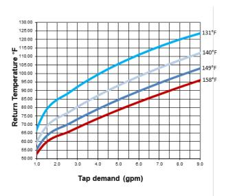
Figure 14: Hydronic return temperatures for HX = B16DW 20 when heating domestic water from 50°F ( $10^{\circ}$ C) to  $120^{\circ}$ F ( $49^{\circ}$ C)
