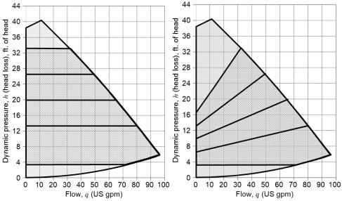
Figure 27: Constant pressure control (L) vs. proportional pressure control (R). It may be necessary, in some cases, to have an external input to the circulator from the system controller to offset (shift) the curves to accommodate peak and seasonal demands through the AquaPorts and HTUs.
