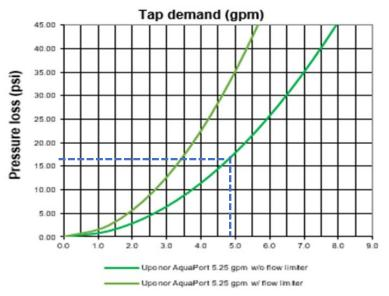
Figure 31: Tap demand pressure loss curve for AquaPort 5.25 U.S. gpm
