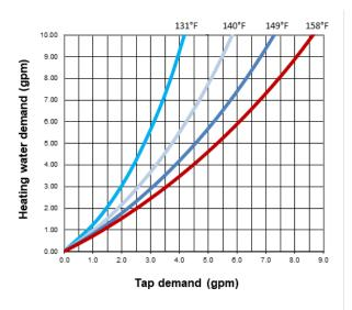
Figure 13: Supply temperatures and flow rates required for HX = B16DW 20 when heating domestic water from 50°F ( $10^{\circ}$ C) to  $120^{\circ}$ F ( $49^{\circ}$ C)
