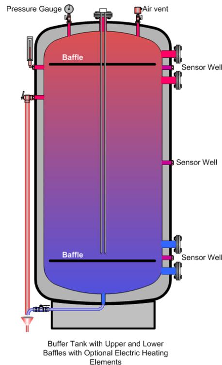
Figure 25: Highly insulated multiport buffer tank with baffles for promoting stratification
