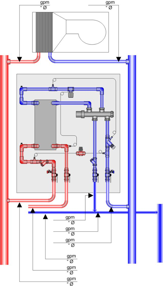
Figure 20: Dimensioning requirements for an AquaPort substation and HTU; includes flow, diameter, velocity, and differential pressure requirements
