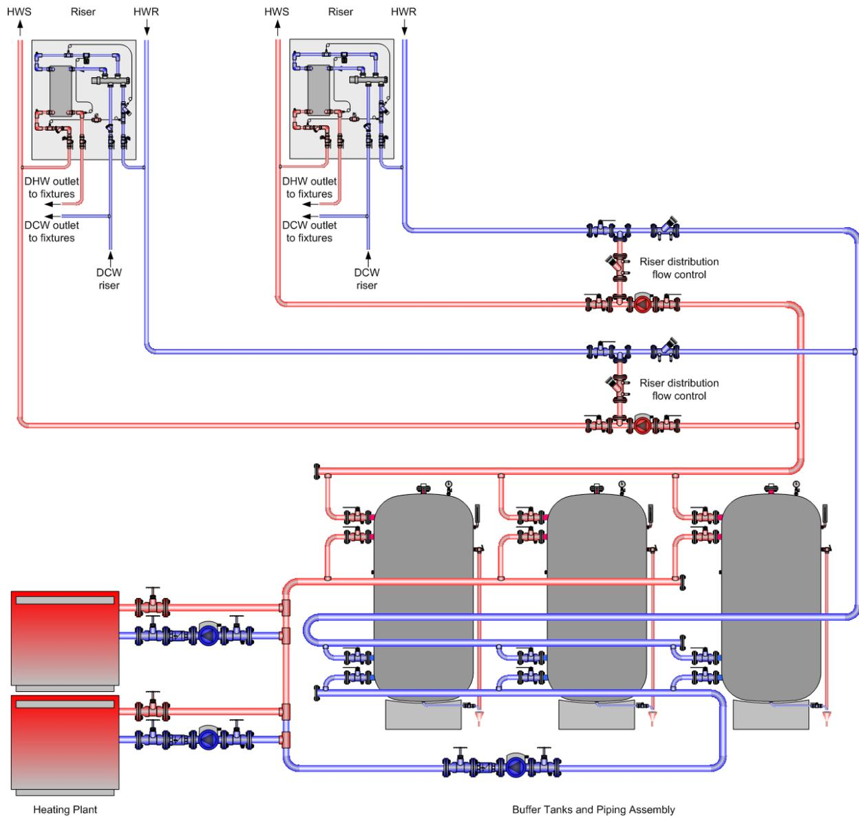
Figure 23: Multisource heating plant using a primary/secondary strategy serving multiple buffer tanks piped in reverse-return, feeding distribution networks to system risers. Generally, parallel buffer tanks are used with systems having more than 200 AquaPort units.
