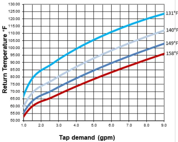
Figure 14: Hydronic return temperatures for HX = B16DW 20 when heating domestic water from 50°F (10°C) to 120°F (49°C)
