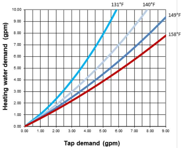
Figure 17: Supply temperatures and flow rates required for HX = B16DW 40 when heating domestic water from 50°F (10°C) to 120°F (49°C)
