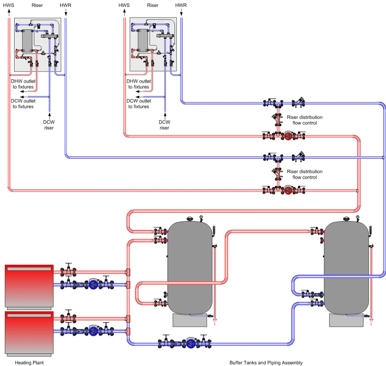
Figure 24: Multisource heating plant using a primary/secondary strategy serving multiple buffer tanks piped in series, feeding distribution networks to system risers. Generally, in-series buffer tanks are used with systems having less than 200 AquaPort units.
