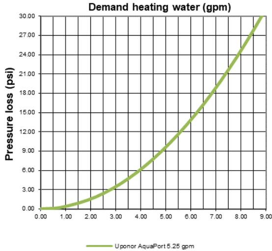
Figure 15: Pressure drop through HX = B16DW 40, on hydronic side (primary) for 5.25 U.S. gpm (1136 L/h) warm-water tapping
