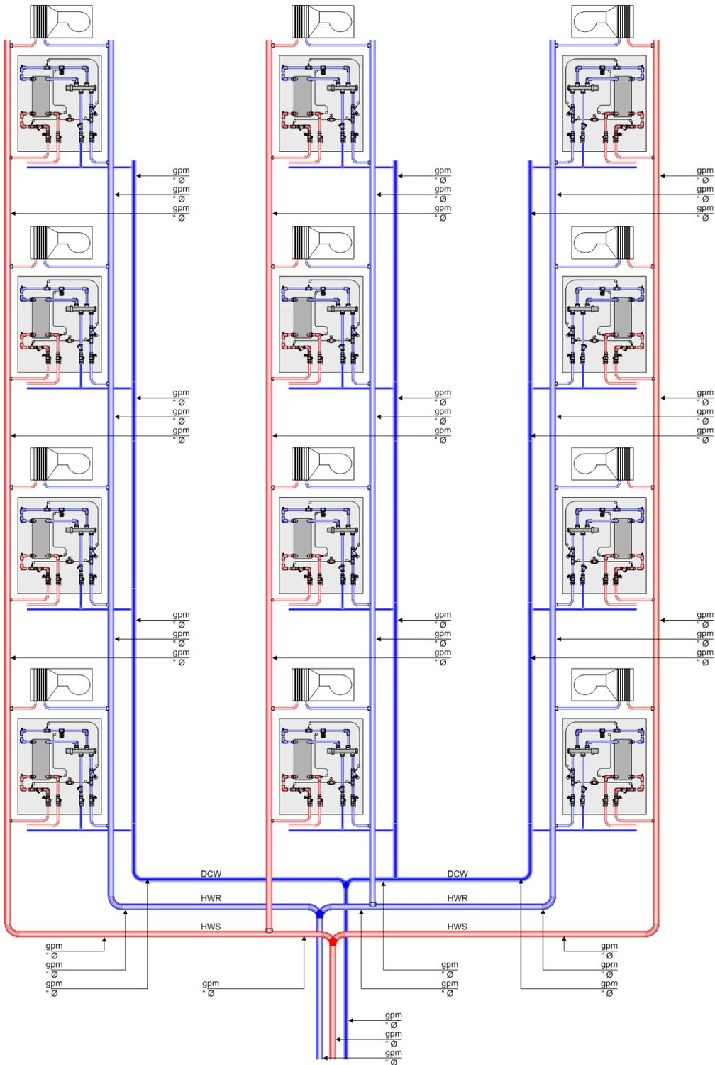
Figure 21: Example of a riser piping layout and dimensioning requirements for an AquaPort system. Note: It is advised that HTUs (i.e., fan coils, radiant floors, radiators, etc.) have return-temperature limiters to prevent unnecessary temperature increases through the heating plant.
