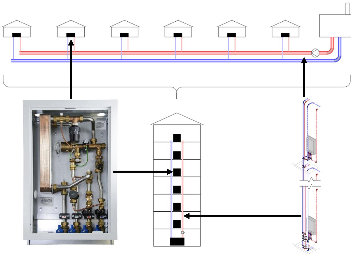
Figure 1: Typical district energy characteristics with heat-transfer stations (top illustration) rearranged into a vertical format (bottom illustration)
