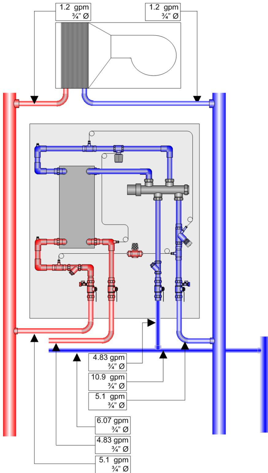
Figure 26: Dimensioning the design flows for the AquaPort
