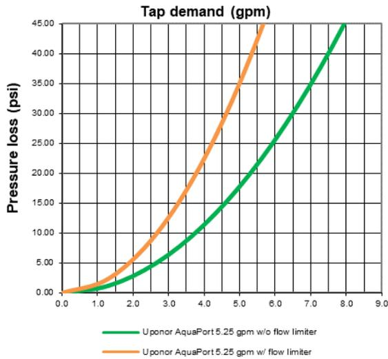
Figure 16: Pressure drop through HX = B16DW 40, on tap water side (secondary) for 5.25 U.S. gpm (19 L/min) warm-water tapping
