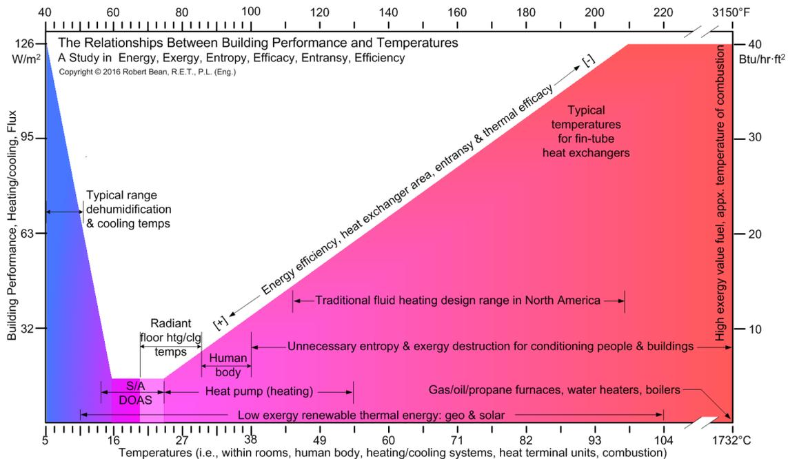
Figure 9: The relationship between building performance (y-axis), heat-exchanger sizing, and temperatures (x-axis). In essence, the larger the heat exchanger surface area to serve lower-flux results in a lower-temperature requirement more aligned with renewable systems, a fundamental principle in sustainability.
