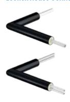
Pre-insulated PE-Xa pipe 90deg elbows with single or twin pipes. Max. load 6 bar /95c. PUR Foam insulation with PE casing
