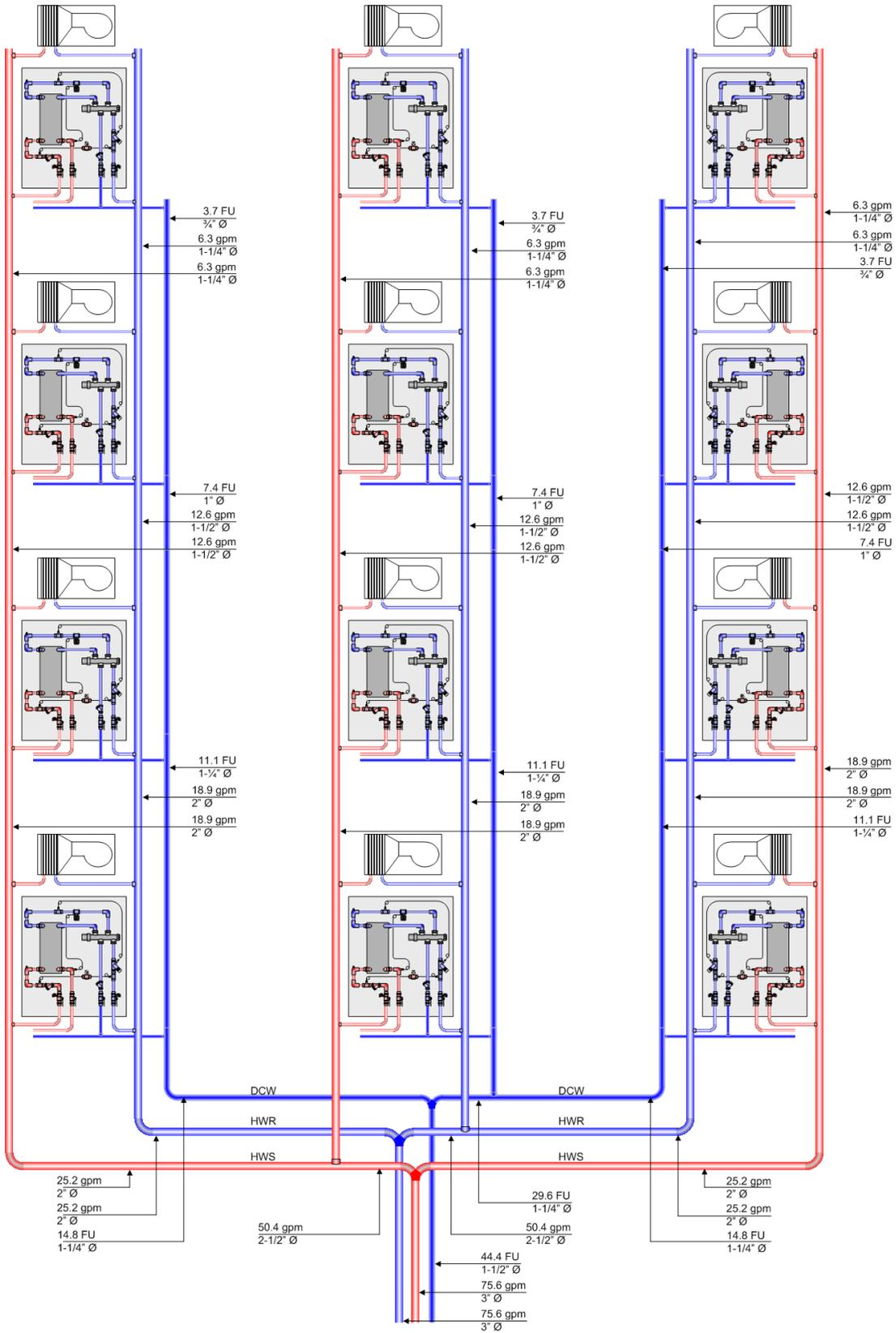
Figure 29: Riser diagram and dimensioning for the example given
