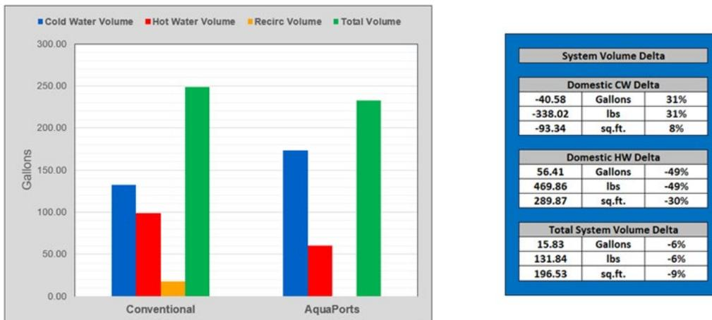
Figure 6: Water volume comparison between a traditional system and an AquaPort system
