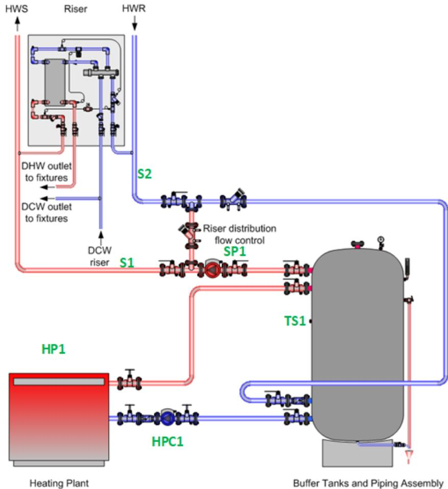
**Figure 26: Typical control points for AquaPorts using buffer tanks**
