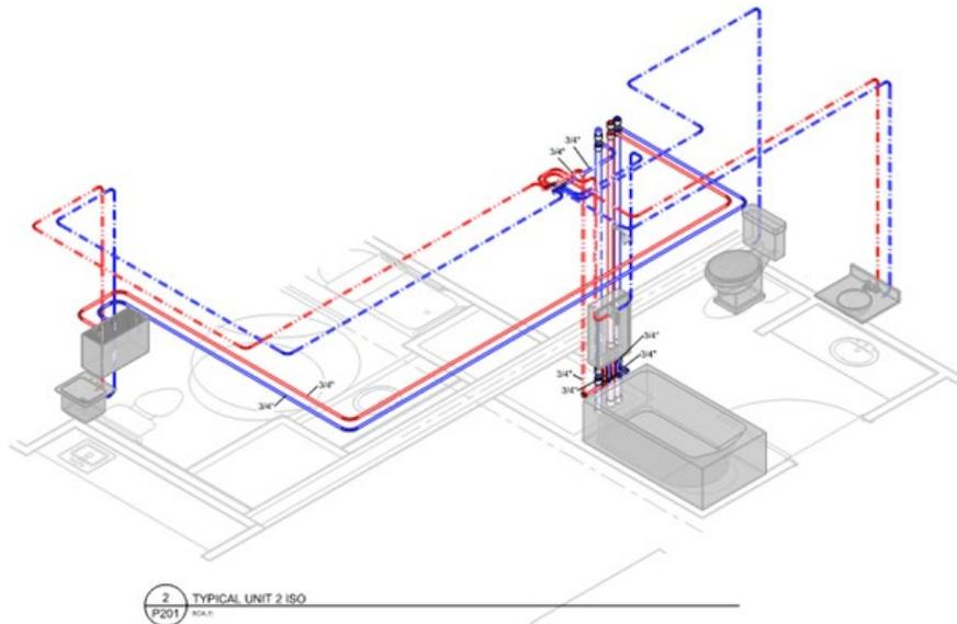
**Figure 28: Typical AquaPort application for lavatory, sink, shower/tub, water closet, and HTU.**
