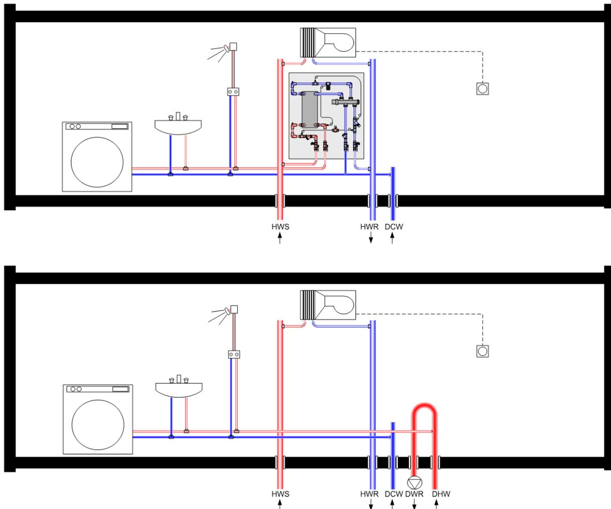
Figure 5: Comparison of sub-stations in a vertical-based district system (top) versus traditional riser piping assemblies (bottom).
