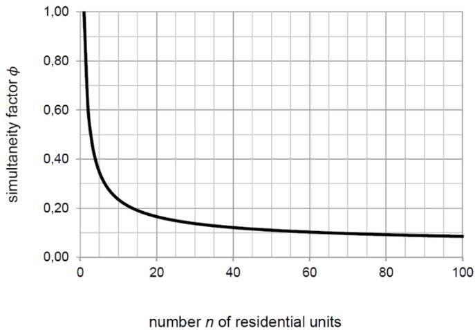
Figure 19: Simultaneity curve representing likelihood of 100% demand on the heating source for domestic purposes based on the number of installed units. See AquaPort sizing example on the following page using the fixture unit method as is standard practice in North America.
