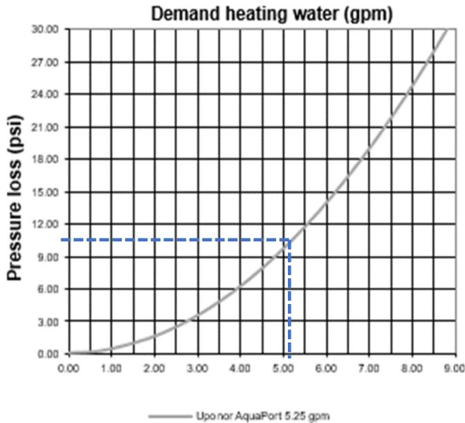
**Figure 30: Demand heating water pressure loss curve for AquaPort 5.25 U.S. gpm**
