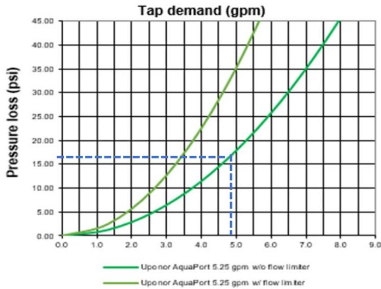
**Figure 31: Tap demand pressure loss curve for AquaPort 5.25 U.S. gpm**
