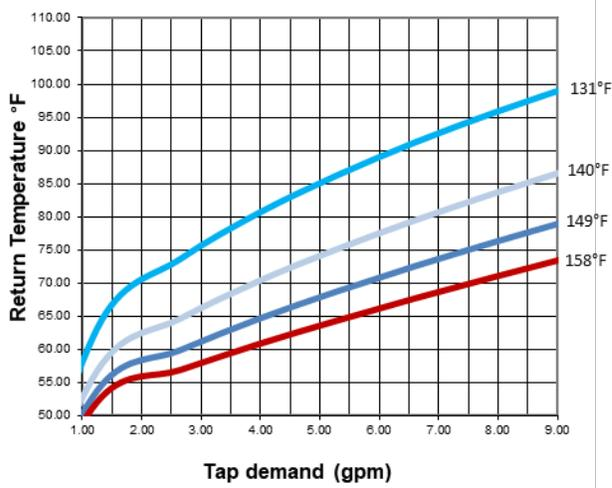
Figure 18: Hydronic return temperatures for HX = B16DW 40 when heating domestic water from 50°F (10°C) to 120°F (49°C)
