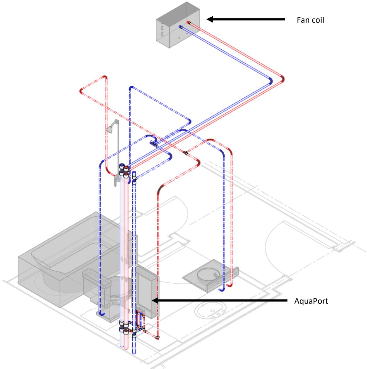
Figure 3: Typical application of an AquaPort sub-station serving the potable requirements of a typical suite. Also shown is the space-heating fan coil (by others).
