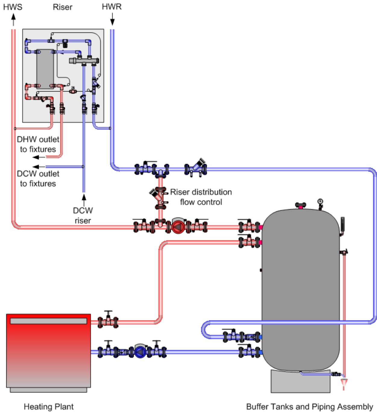
Figure 22: Single-source heating plant with a buffer tank feeding distribution network to system risers.
