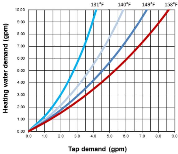
Figure 13: Supply temperatures and flow rates required for HX = B16DW 20 when heating domestic water from 50°F (10°C) to 120°F (49°C)
