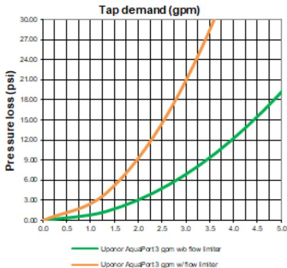
Figure 12: Pressure drop through HX = B16DW 20, on tap water side (secondary) for 3 U.S. gpm (11.4 L/min) warm water tapping
