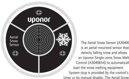
The Aerial Snow Sensor (A3040095) is an aerial-mounted sensor that detects falling snow and allows an Uponor Single-zone Snow Melt Control (A3040654) to automatically start the snow melting equipment. System stop is provided by the control's
