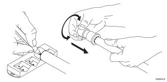
2. Press the fitting onto the pipe with the appropriate tool and visually check the result.
