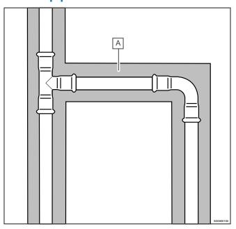
Chased pipes must not be in direct contact with the plaster, but wrapped in a pad of elastic material, such as glass wool or plasticfoam (A). Thus fitted, soundproofing requirements can also be satisfied, but always refer to local guidelines and regulations.
