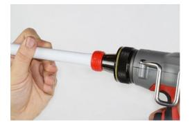
5. Remove the tool from the end of the pipe, and immediately insert the Q&E fitting, pushing the pipe until the ring sits against the pipe stop
