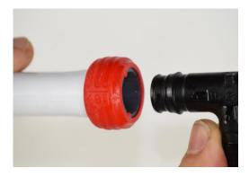
6. The pipe and ring will now contract around the Q&E fitting and the joint will be watertight in around 10 – 15 seconds
