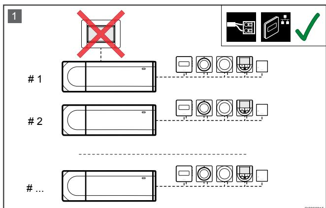
Connect and register thermostats, and system devices, to the controllers.
