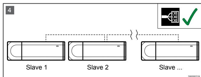
Connect the controllers to each other using the Base PRO controller system device bus.
