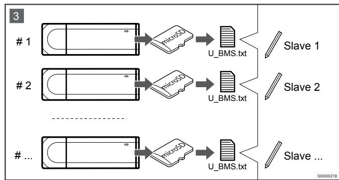
Edit the U\_BMS.txt file, on the controller microSD card, to setup the controller Modbus RTU interface.
