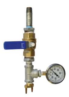
Figure 1: Flow test assembly
