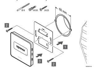
Attach the thermostat to the wall using the wall bracket, screws and wall plugs.
