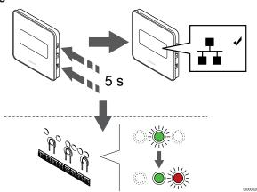
Press and hold both  $\blacktriangle$  and  $\blacktriangledown$  buttons on the thermostat until the text **CnF** (configure) and a communication icon is displayed.
