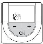
Use buttons - or + to change the value, press the OK button to set the value and move to the next editable value.
