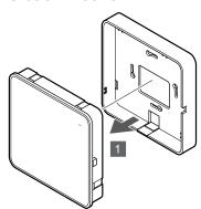
Separate the communication module from its removable back mount.
