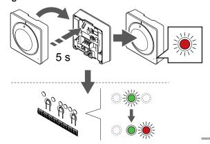
Gently press and hold the registration button on the thermostat, release when the LED on the front of the thermostat starts flashing.
