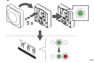
Gently press and hold the registration button on the thermostat, release when the LED starts flashing green (located in the hole above the registration button).
