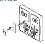
Label the thermostat, where suitable, with the channel numbers they are to control, for example, #02, #03. For a system with several room controllers, add the ID of each room controller, for example, 1.02, 1.03, 2.02, 2.03.
