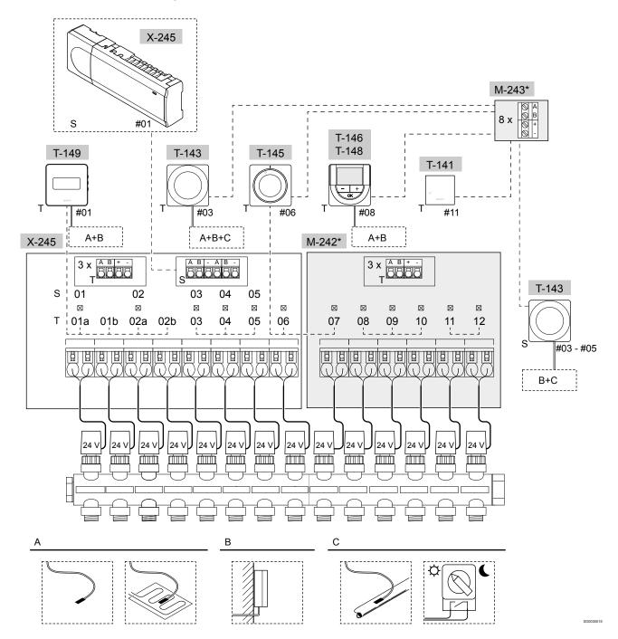
\*) This example contains optional accessories which adds six actuator outputs (slave module M-242) and extra bus connectors (slave module M-242 and star module M-243) to the Uponor Smatrix Base Pulse controller
