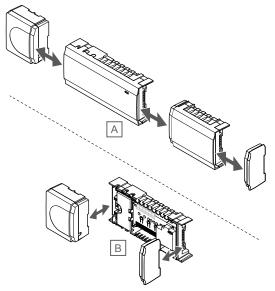
The room controller is designed with the option of modular placement in mind. This means that all major parts are detachable and can be placed separately (some extra wiring may be required depending on placement).
