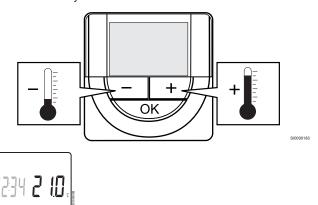
To adjust the thermostat temperature setpoint of the current control mode:
