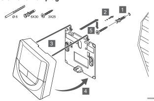
Attach the thermostat to the wall using the screw and wall plug.
