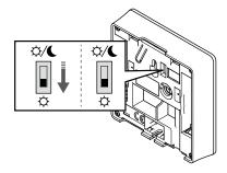
Optional: If tamper alarm was activated during registration, set the Disable timer switch to preferred mode.
