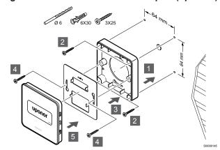
Attach the thermostat to the wall using the wall bracket, optional surface adaptor, screws and wall plugs.
