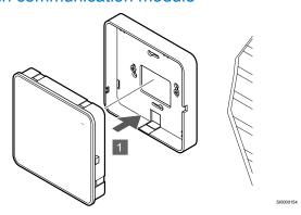
Attach the communication module to the removable back mount.
