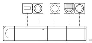
The star module is attached to the room controller and slave module (if available) adding extra connection terminals to the system. Each thermostat in the example is connected direct to the room controller, slave module (if available) and star module.
