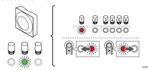
Use buttons < or > to move the pointer (LED flashes red) to a preferred channel.
