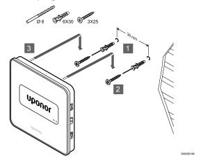
Attach the thermostat to the wall using the screw and wall plug.
