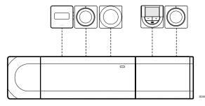
Every thermostat in the example is connected to the room controller and slave module (if available) with its own cable.
