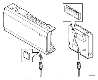
Connect the supplied communication cable to the communication module and room controller.
