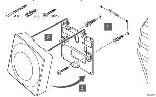
Attach the thermostat to the wall using the wall bracket, screws and wall plugs.
