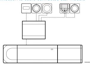
The star module is connected to the room controller and/or slave module (if available) with a cable, using two of the extra connection points. Each thermostat in the example is connected direct to the star module, except one that is connected with daisy chain.
