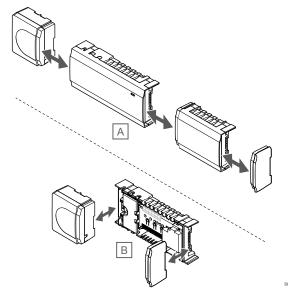
The components can either snap on or off without the need of removing the covers (A, recommended to do on a flat surface or on a DIN-rail), or by sliding them into place when the covers are removed
