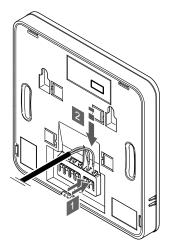
1. Press the push buttons on the connection terminals.
