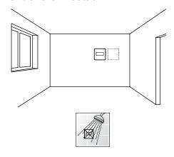
Ensure that the thermostat is away from any source of humidity and water splashes (IP20).
