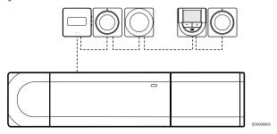
The thermostats in the example are connected in series and only one cable needs to be routed from the room controller and slave module (if available).
