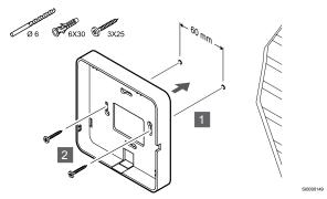
Attach the communication module back mount to the wall using the screws and wall plugs.
