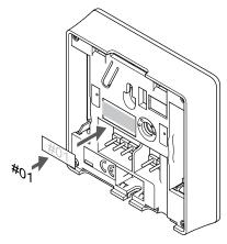
Label the thermostat, where suitable, with the channel numbers they are to control, for example, #S02, #S03.
