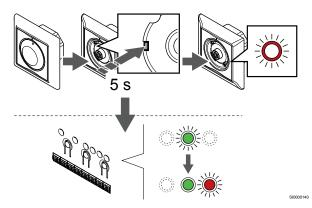
Using a pointed instrument, gently press and hold the registration button on the thermostat, release when the LED above the dial starts flashing.
