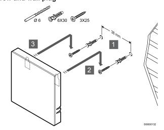
Attach the thermostat to the wall using the screw and wall plug.
