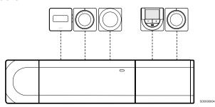
Every thermostat in the example is connected to the room controller and slave module (if available) with its own cable.
