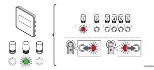
Use buttons < or > to move the pointer (LED flashes red) to a preferred channel.
