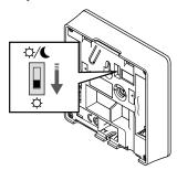
Optional: To activate tamper alarm for the thermostat, set the Disable timer switch to Comfort mode (\$\square\$) before registering the thermostat.
