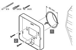
Attach the communication module back mount to the wall box.
