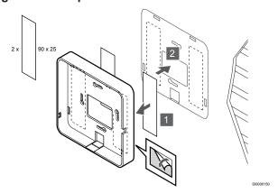
Attach the communication module back mount to the wall using adhesive tape.
