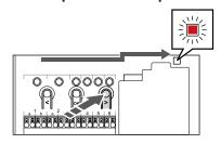
Use buttons < or > to move the pointer to the power LED (LED flashes red).
