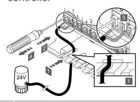
Each thermostat can control one or more channels. To simplify installation and maintenance, Uponor recommends that actuators controlled by the same thermostat shall be wired in sequence to the channels.
