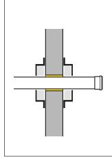
Wall Mounting (fire protection collar required on both sides)
