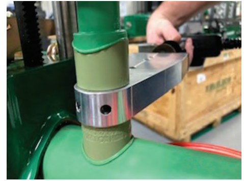
Figure 2-8: Heating a saddle outlet
