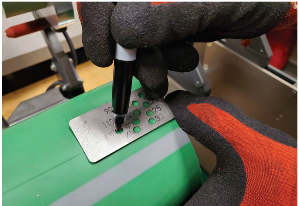
Figure 2-2: Mark weld depth
