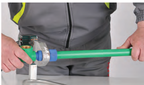
Figure 2-3: Heating the pipe and fitting
