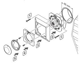
To attach thermostat T-144 to the wall:
