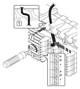
To connect a communication cable to a star module:
