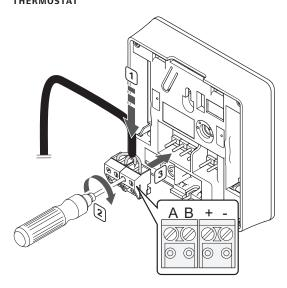
To connect a communication cable to a timer:
