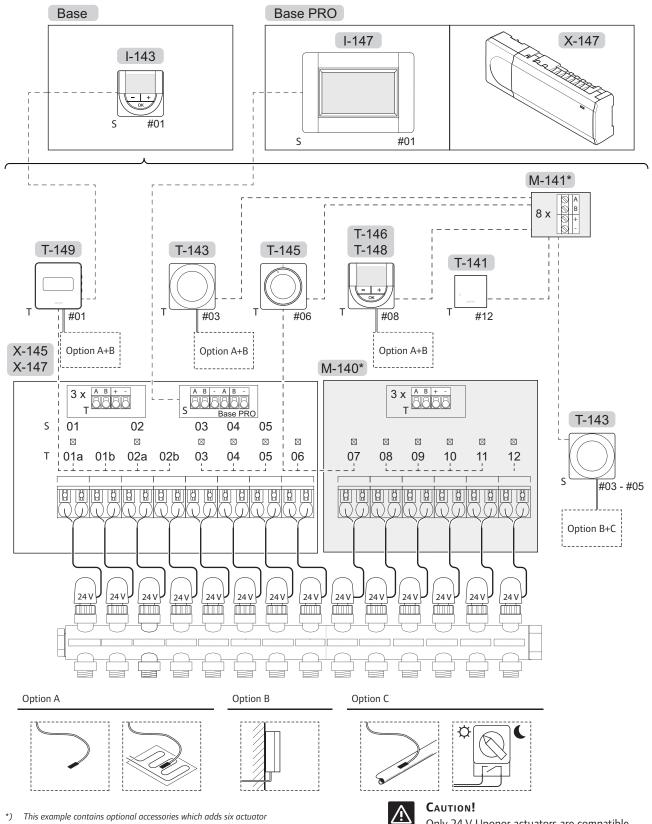
outputs (slave module M-140) and extra bus connectors (slave module M-140 and star module M-141) to the Uponor Smatrix Base controller
