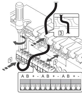
To connect a communication cable to the controller:
