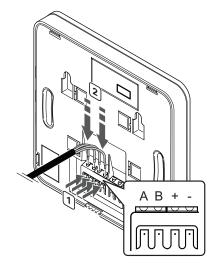
To connect a communication cable to thermostat T-149:
