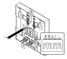
To connect a communication cable to thermostat T-149:
