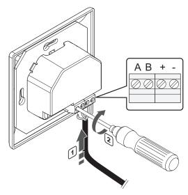
To connect a communication cable to thermostat T-144:
