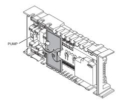
To connect a circulation pump to the controller:
