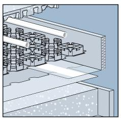
Figure 5: Proper edge strip location
