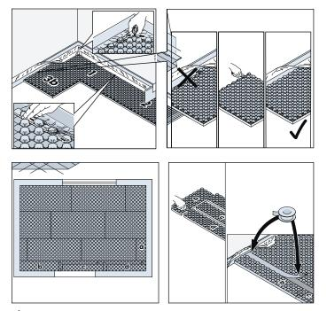
Figure 15: Use duct tape to seal gaps between panels
