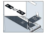
Figure 14: Fit panels to floor area
