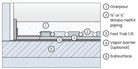
Figure 10: Fast Trak 1.3i installation application
