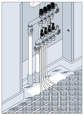
Figure 9: Connect piping to manifold
