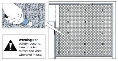
Figure 7: Fit panels to floor area
