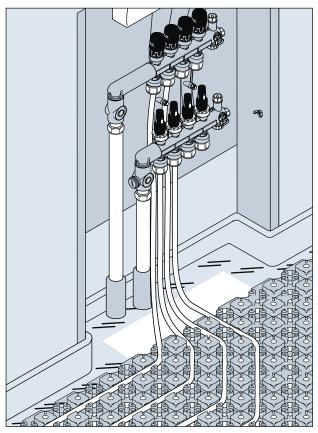
Figure 17: Connect piping to manifold
