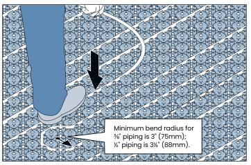
Figure 16: Install piping
