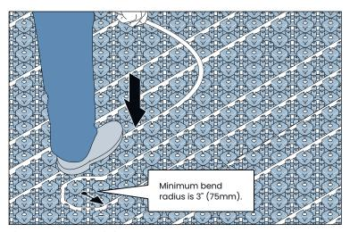
Figure 8: Install piping
