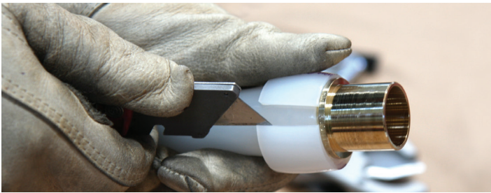
Figure 2-34 : Retirer la bague
