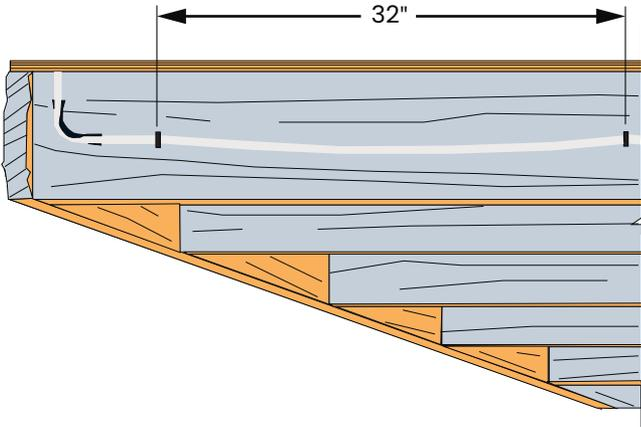
**Figure 9-11: Horizontal pipe support spacing**
