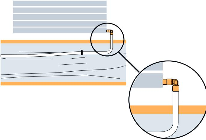
**Figure 9-6: Connecting Uponor PEX with ProPEX baseboard elbows**
