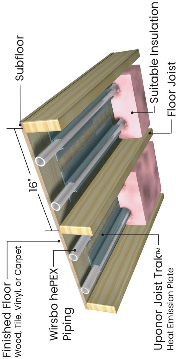
**Figure 7-18: Joist heating using Joist Trak panel**
