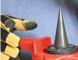
**Figure 4-11: FORCE LOGIC expansion head installation**
