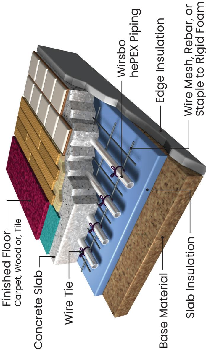
**Figure 7-7: Slab on or below grade with under-slab and edge insulation**
