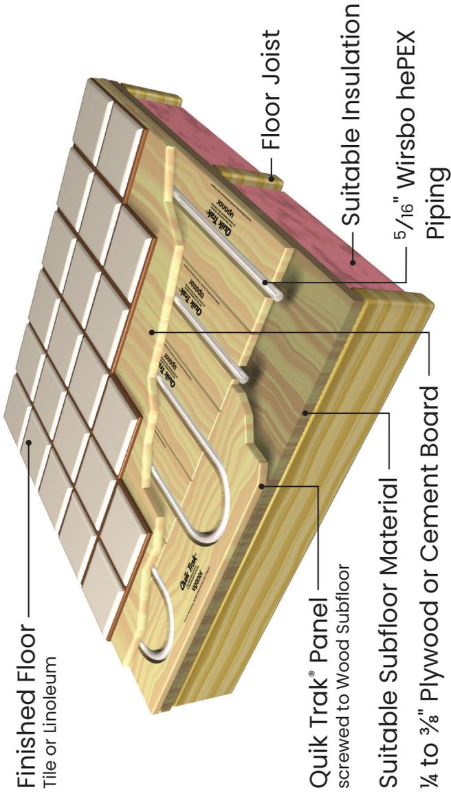
**Figure 7-21: Quik Trak over a wood subfloor with tile/linoleum floor covering**
