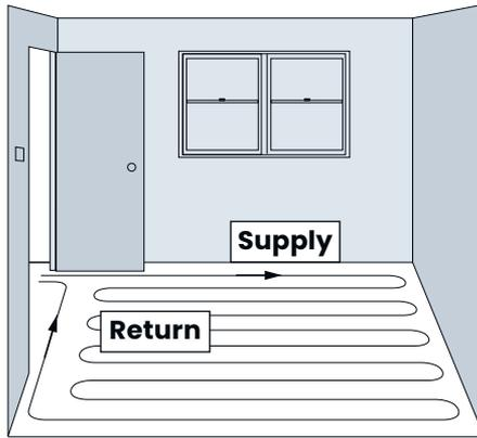
**Figure 6-1: Single-wall serpentine** — Use when a single wall represents the major heat loss of the zone. The supply is fed directly to the high heat loss wall and then serpentine toward the lower heat loss area. Start piping runs 6" from walls or nailing surfaces. A 6" on-center piping run is often installed along outside walls to improve response time.
