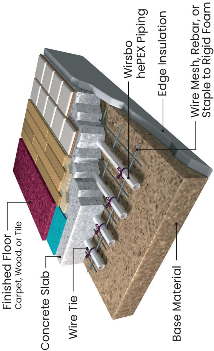
**Figure 7-6: Slab on or below grade over a compacted soil/sandbed**
