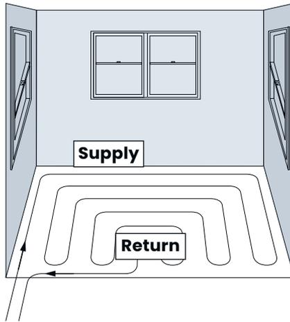
**Figure 6-3: Triple-wall serpentine** — Use when there are three walls representing the major heat loss of the room. The supply is fed along the heat loss walls in an alternating pattern and serpentine toward the lower heat loss area of the room. Start piping runs 6" from walls or nailing surfaces. A 6" on-center piping run is often installed along outside walls to improve response time.
