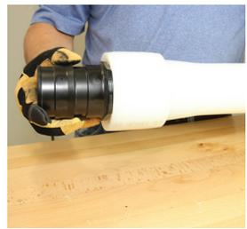
**Figure 4-20: Insert fitting**
