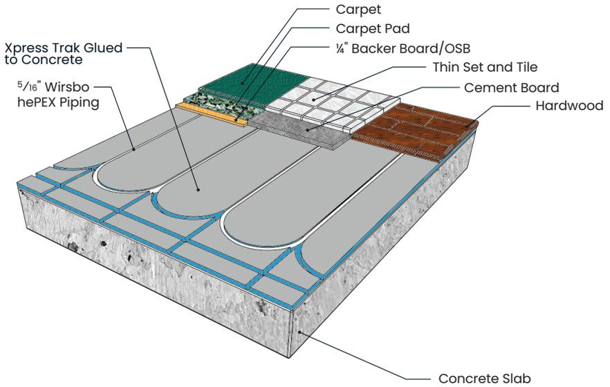
**Figure 7-14: Xpress Trak over a concrete floor**
