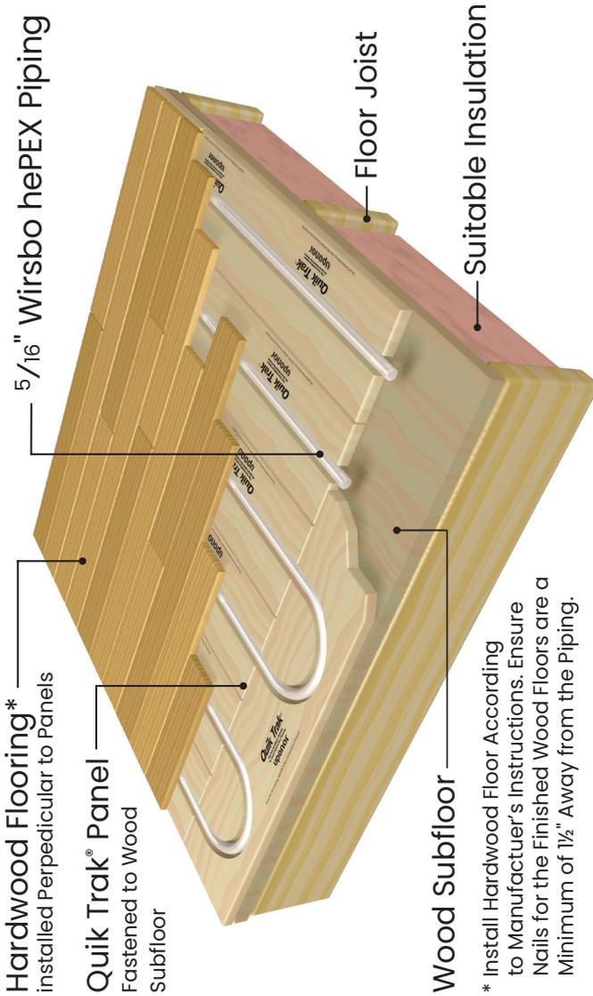
**Figure 7-20: Quik Trak over a wood subfloor with hardwood floor covering**
