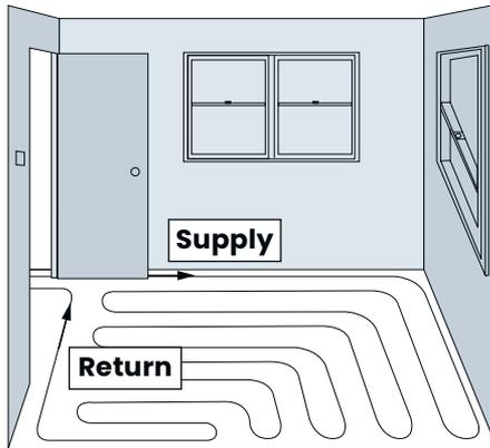
**Figure 6-2: Double-wall serpentine** — Use when there are two adjacent walls representing the major heat loss of the room. The supply is fed directly to either of the heat loss walls and then serpentine toward the lower heat loss area in an alternating pattern against the two heat loss walls. Start piping runs 6" from walls or nailing surfaces. A 6" on-center piping run is often installed along outside walls to improve response time.
