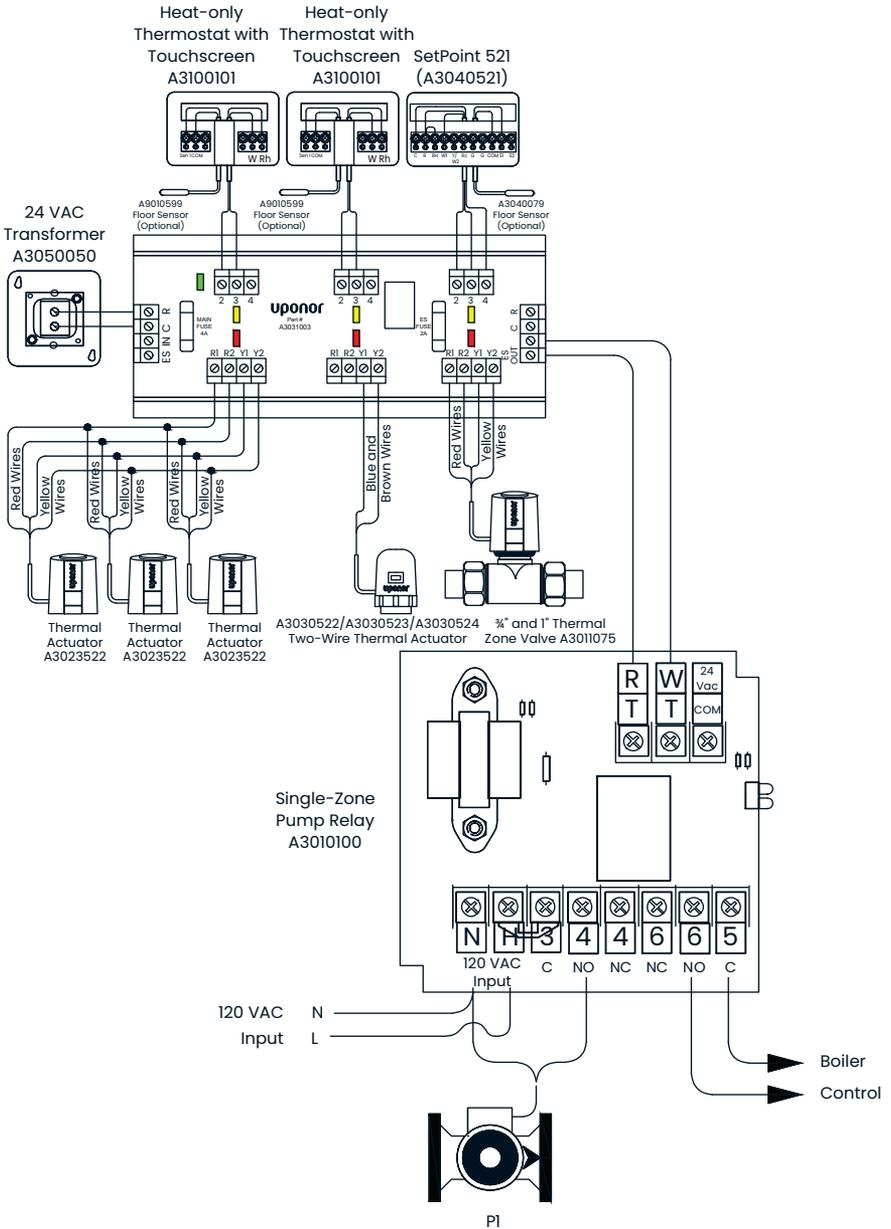
Figure 9-5: Zone Control Module and pump relay
