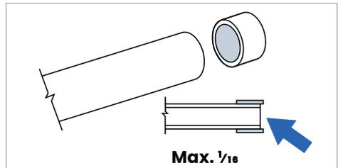
**Figure 4-23: Slide the expanded ring over the end of the piping**
