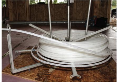
**Figure 3-1: PEX Uncoiler**
