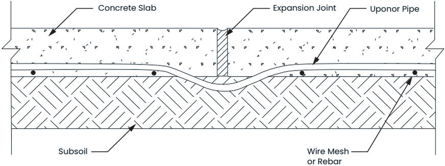
**Figure 7-3: Dip piping below slab into subsoil**
