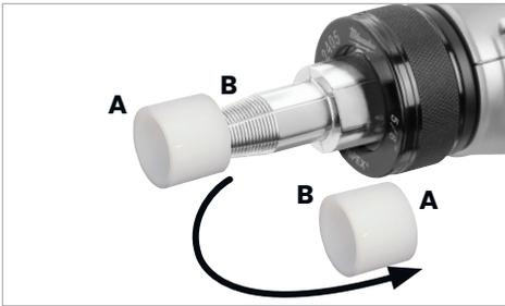
**Figure 4-22: Expand each side of the ring**
