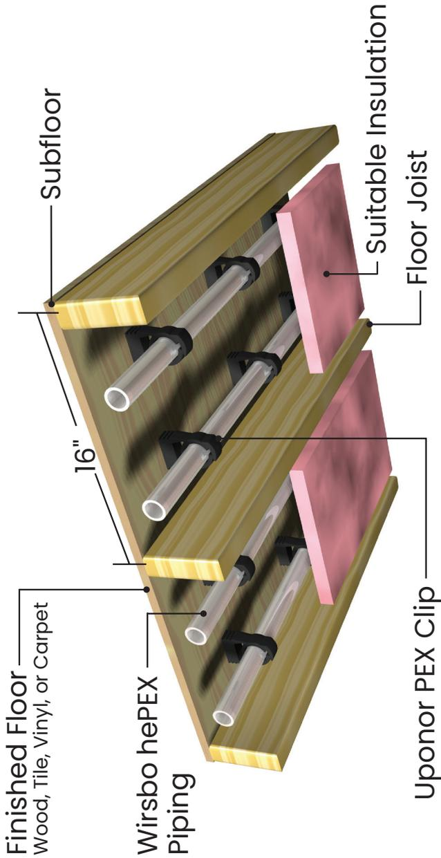
**Figure 7-19: Joist heating using PEX clips**
