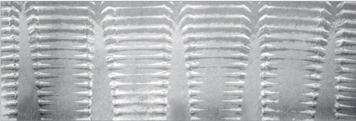
**Figure 4-32: Expansion without proper rotation**
