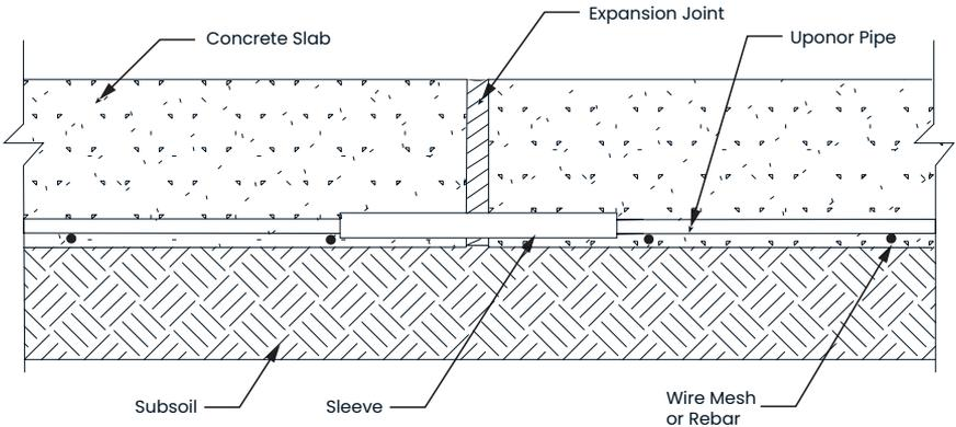
**Figure 7-4: Wrap with a pipe sleeve or larger-diameter pipe**
