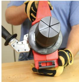
**Figure 4-14: Correct expansion head alignment**
