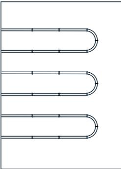
**Figure 7-9: Slab on or below grade – single pour over piping in a sandbed**
