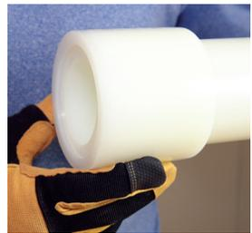
**Figure 4-17: Ensure ring reaches stop edge**
