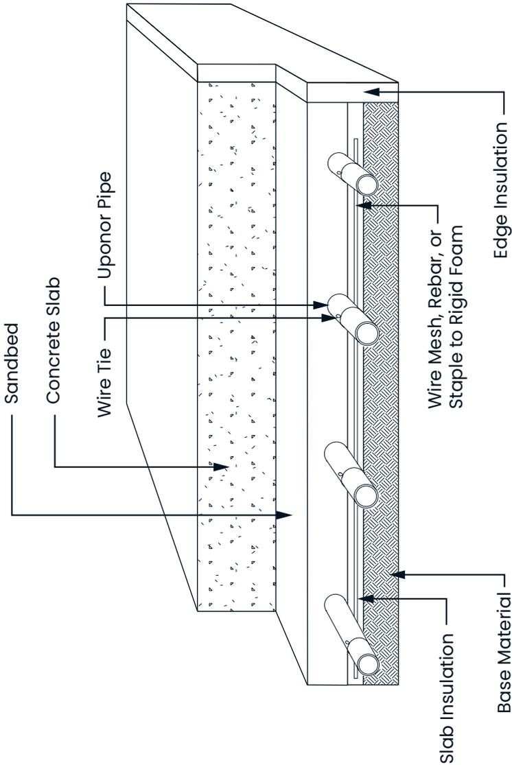
**Figure 7-8: Slab on or below grade – single pour over piping in a sandbed**
