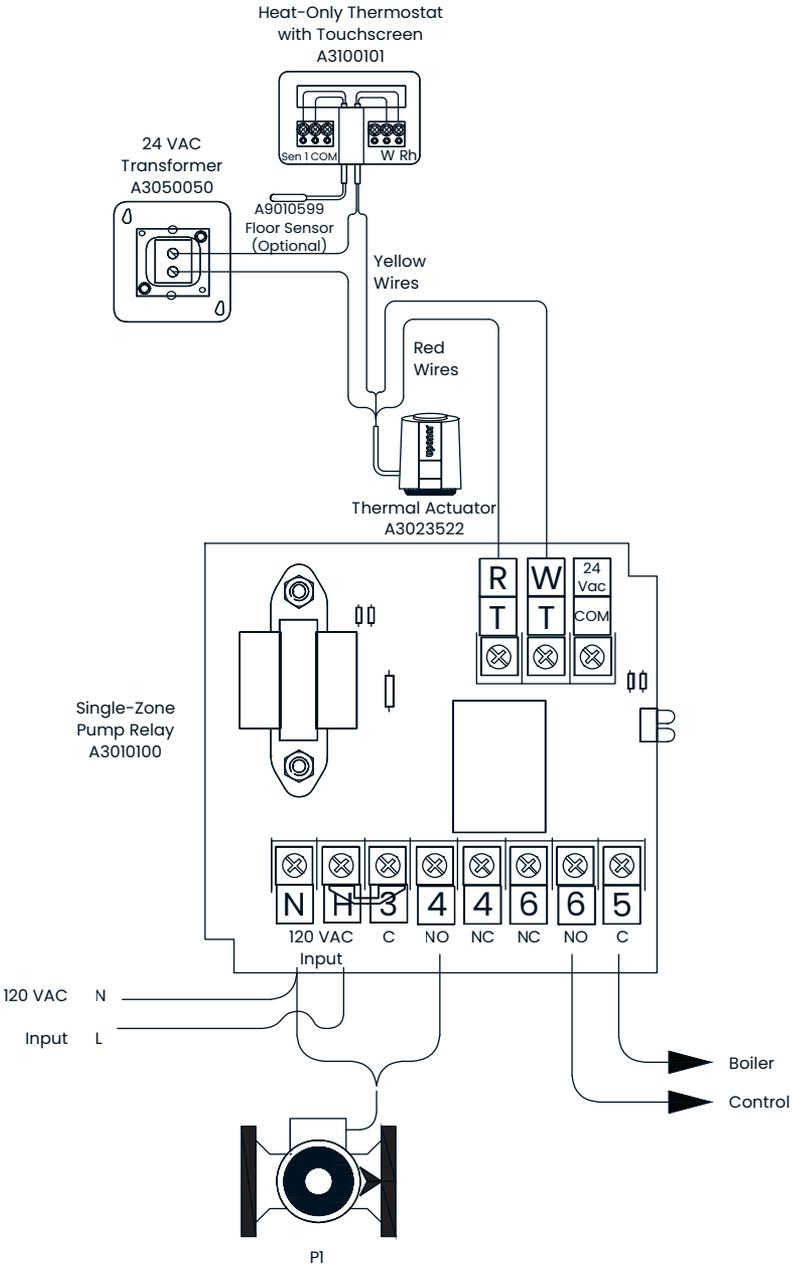
Figure 9-3: Heat only with actuator and pump relay
