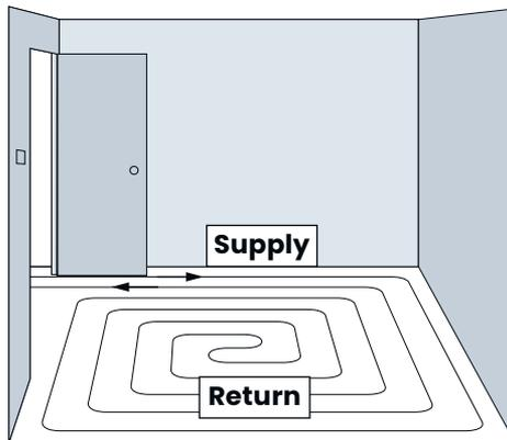
**Figure 6-4: Counter flow** — Use when the heat loss for the room is evenly distributed throughout the entire room or the major heat loss is to the floor. The supply is fed along the exterior of the room spiraling inward with the return paralleling it from the center of the room. Start piping runs 6" from walls or nailing surfaces. A 6" on-center piping run is often installed along outside walls to improve response time.
