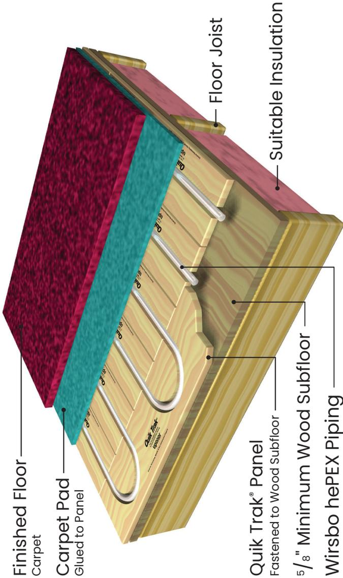
**Figure 7-22: Quik Trak over a wood subfloor with carpet floor covering**
