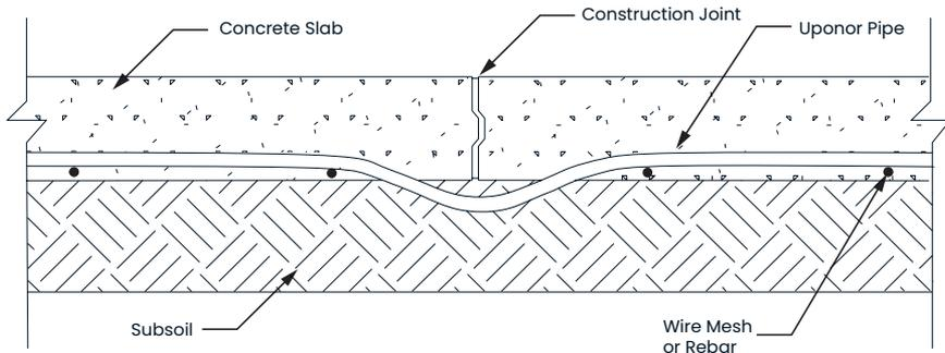
**Figure 7-1: Construction joint – Two pours completed at different times**
