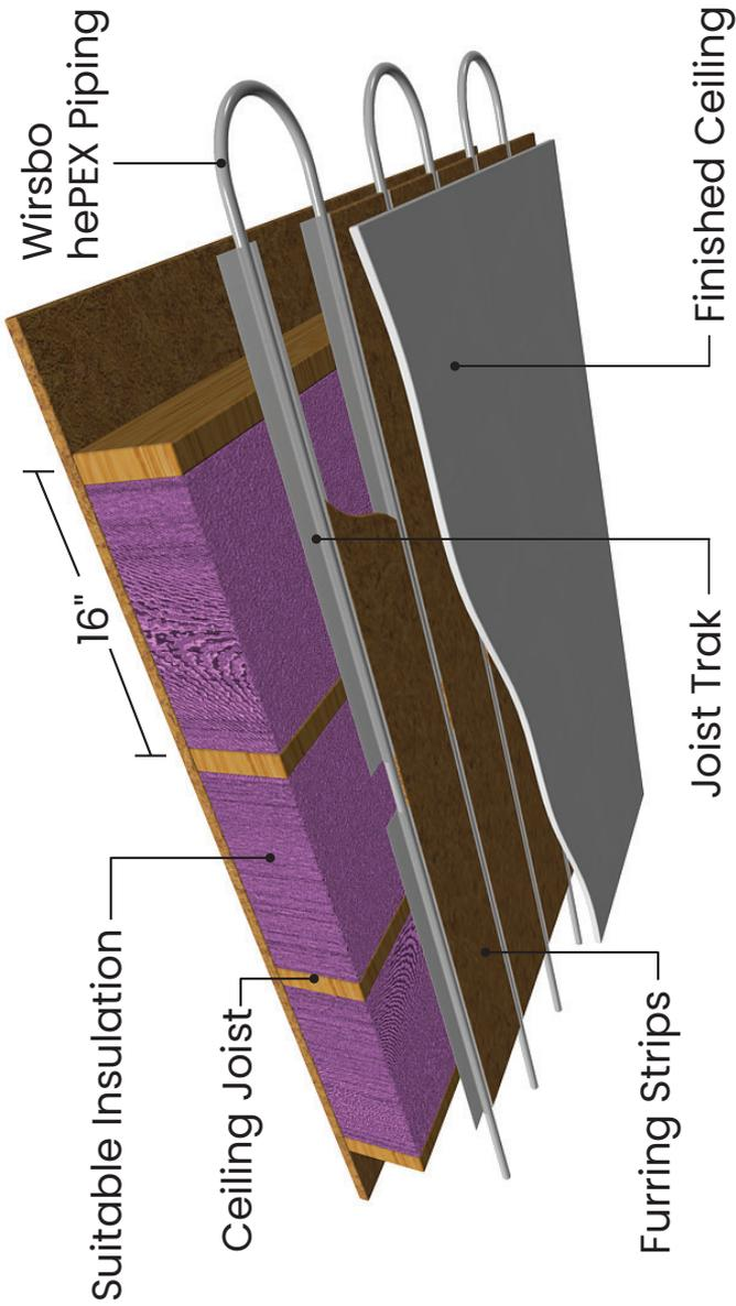
**Figure 7-25: Radiant ceiling using Joist Trak panel**
