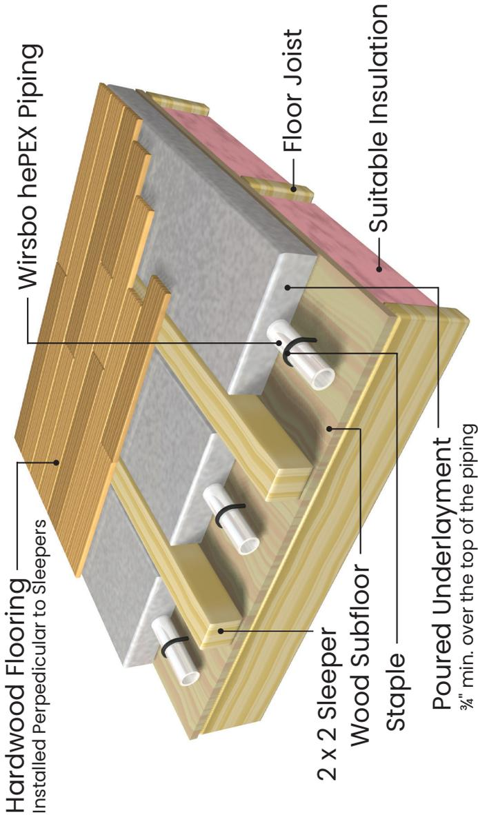
**Figure 7-11: Poured underlayment with sleepers over a suspended wood subfloor**
