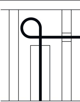
Figure 7-26: Single-plate expansion loop
