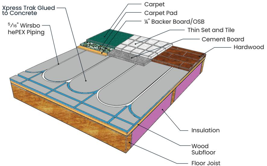
**Figure 7-15: Xpress Trak over a suspended floor**
