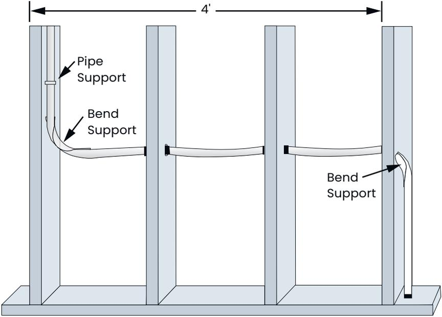
**Figure 9-10: Allow  $\frac{1}{8}$ " to  $\frac{3}{16}$ " of slack per foot of Wirsbo hePEX pipe ( $4' \times \frac{3}{16}" = \frac{3}{4}"$  of slack)**
