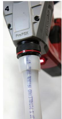
**Figure 4-10: Expansion with Milwaukee M18 ProPEX Expansion Tool**
