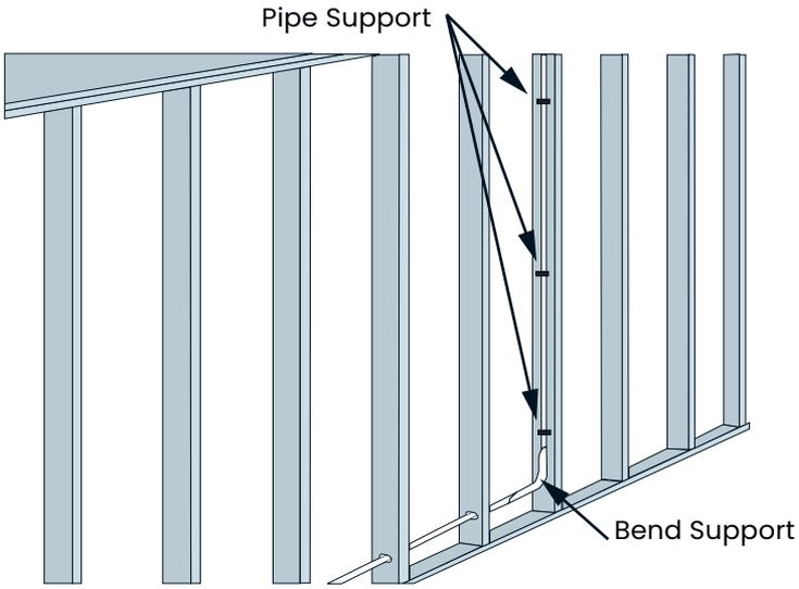
**Figure 9-12: Vertical pipe support spacing**
