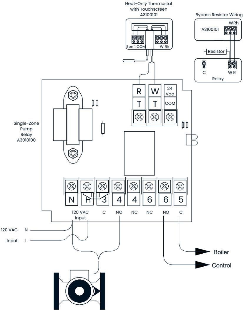
**Figure 9-2: Heat only and pump relay**
