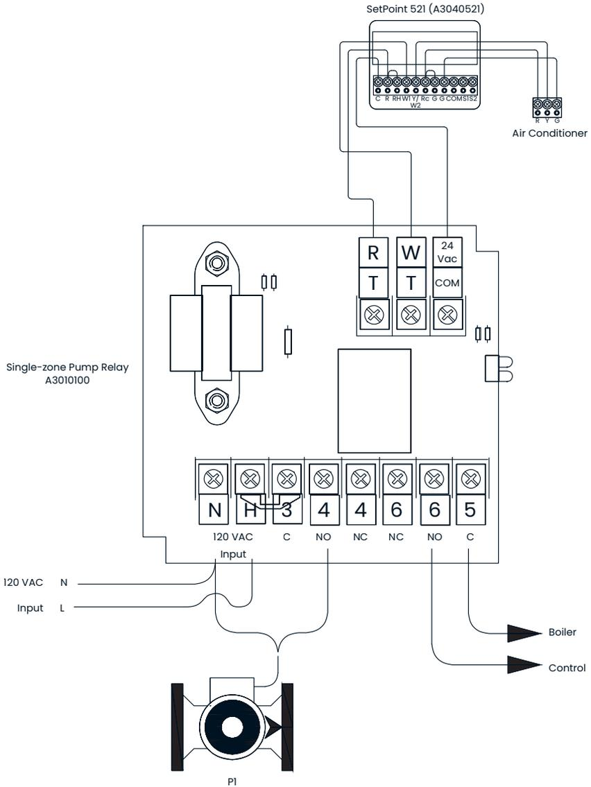
**Figure 9-4: SetPoint 521 and pump relay**
