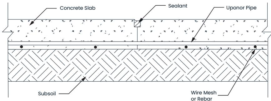
**Figure 7-2: Control joint – Sawed or formed (allows concrete to crack in a predictable pattern)**
