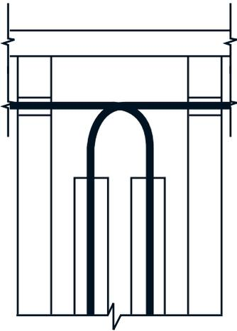
Figure 7-27: Double-plate expansion loop
