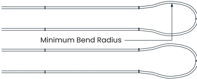
**Figure 3-3: Minimum bend radius**
