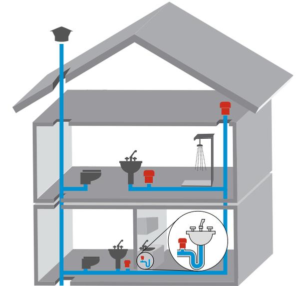
Air admittance valves are ideal for installation at the ends of non-ventilated risers and near sanitary fixtures located at a considerable distance from the riser.
