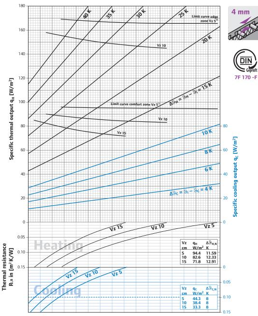
Design diagram heating/cooling Uponor Minitec with 15 mm levelling layer ( $s_{ii} = 4 \text{ mm}$  with  $I_{ii} = 1.0 \text{ W/mK}$ )
