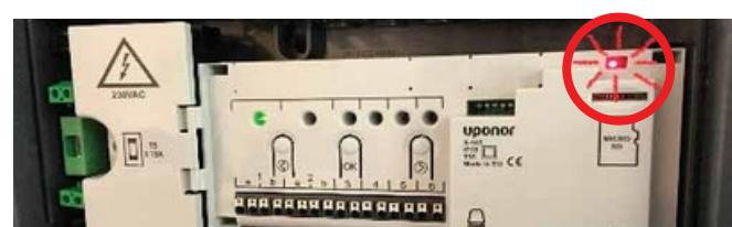
4. Press the OK button on the controller to select device registration. Channel 1 starts flashing red. Press the OK button on the controller again to select system device channel 1. Channel 1 LED starts flashing green.
