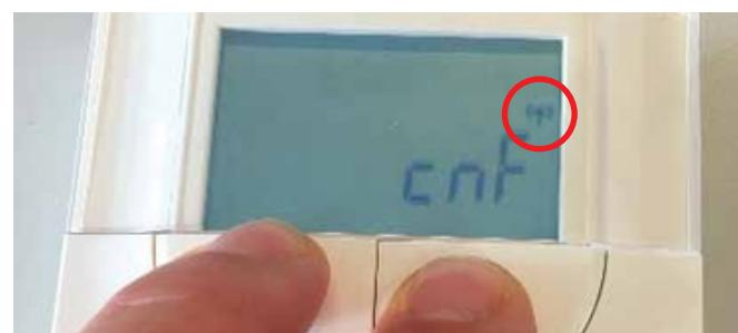
5. On the Timer press and hold both the + and - buttons until you see **cnf** and keep them pressed until the communication icon on the display screen appears.
