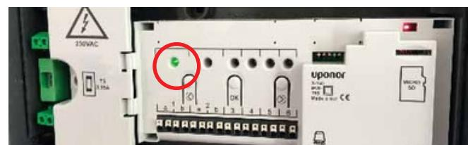
6. The channel 1 LED on the controller will now be fixed green which shows the registration of the timer (system device) was successful.
