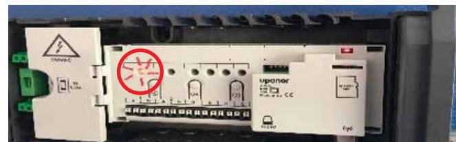
3. Move the red flashing LED to the power LED using the < or > right buttons. The power LED will start to flash.
