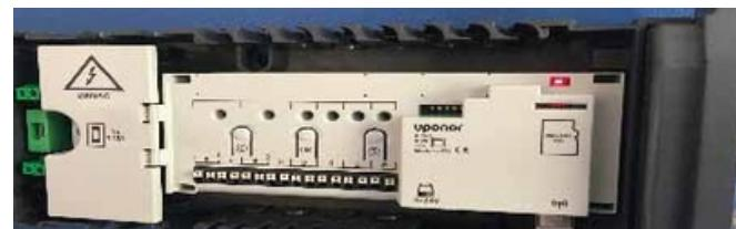
2. Press and hold the OK button on the controller until the LED for the first unregistered channel begins to flash.
