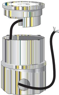
Automatic start and stop operation requires the installation of a Pavement Snow and Ice Sensor (A3040090). The control continually monitors the sensor for the presence of moisture and slab temperature conditions in which snow or ice may be present. When moisture is detected, the control will show Sensor Water Wet in the View menu. When the sensor is dry the control will show Sensor Water Dry. The control includes a
