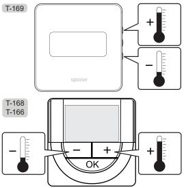
To adjust the thermostat temperature setpoint of the current control mode:
