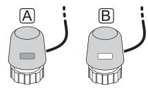
Actuator has closed the valve - empty indicator А
