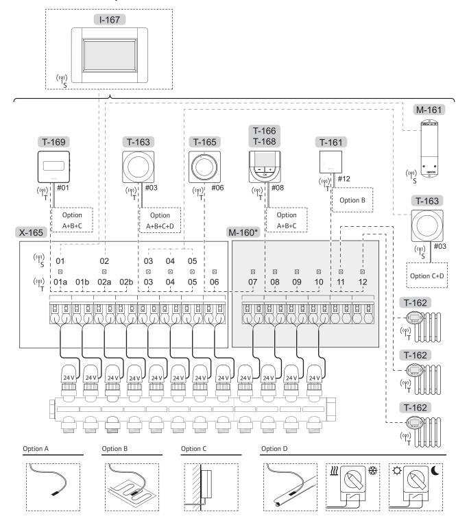
\*) This example contains optional accessories which adds six actuator outputs (slave module M-160) to the Uponor Smatrix Wave controller
