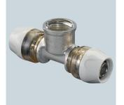
Uponor RTM tee – with inner thread – with integrated pressing function, pressed state identification and colour coding, cylindrical inner thread to ISO.
