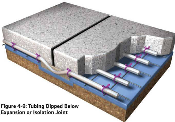
Figure 4-9: Tubing Dipped Below Expansion or Isolation Joint
