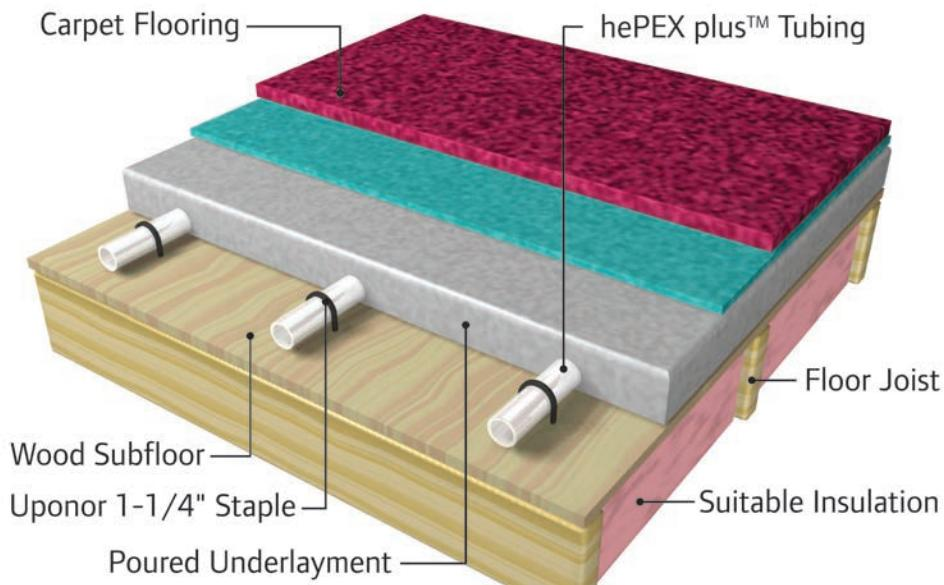
Figure 4-7: Slab on Wood Subfloor
