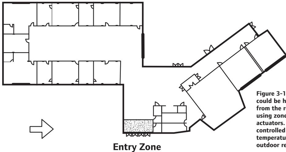
**Figure 3-14:** An entry area could be hydraulically isolated from the rest of the system by using zone valves or thermal actuators. This zone could be controlled so the supply water temperature is reset based on outdoor relative humidity.
