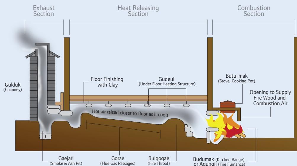
**Figure 1-1: An ondol, also called gudeul, in Korean traditional architecture. This type of underfloor heating uses direct heat transfer from wood smoke to the underside of a thick masonry floor.**
