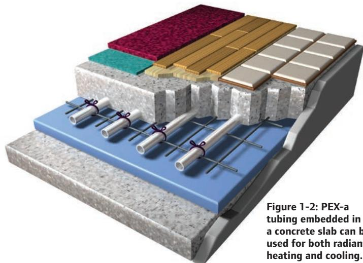
**Figure 1-2:** PEX-a tubing embedded in a concrete slab can be used for both radiant heating and cooling.
