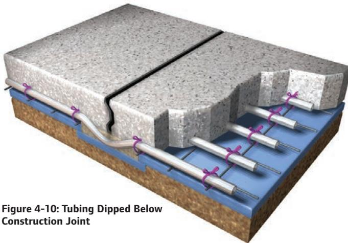
Figure 4-10: Tubing Dipped Below Construction Joint
