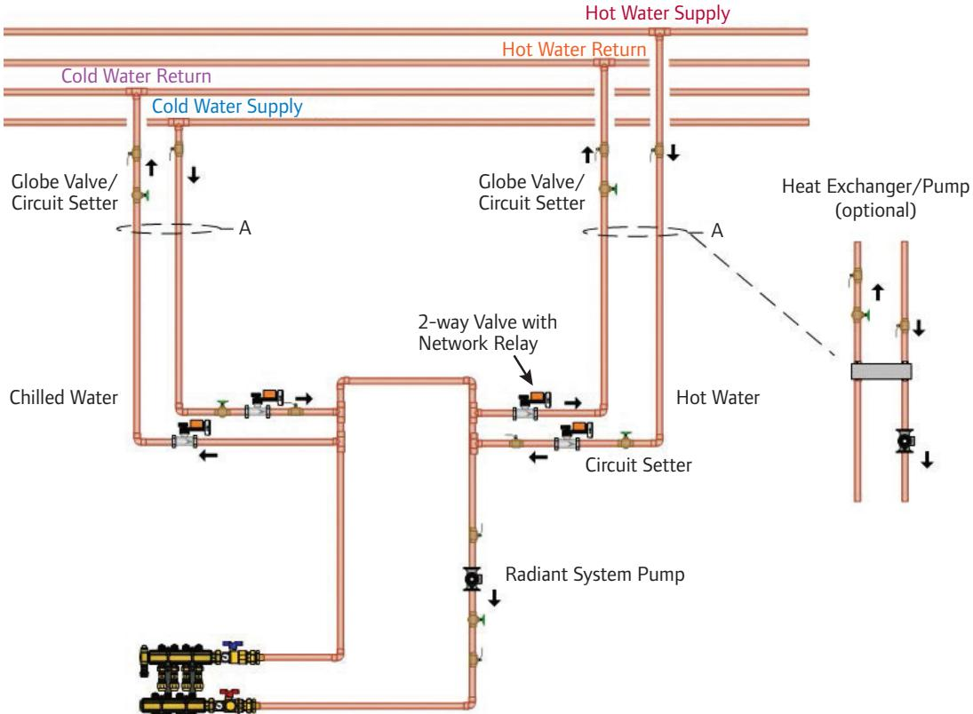
**Figure 3-2: Local Secondary Injection System Using Two-way Valves**
