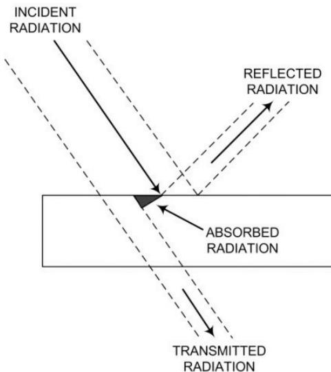
**Figure 2-2: Reflection, Absorption and Transmission of Short-wave Radiation**
