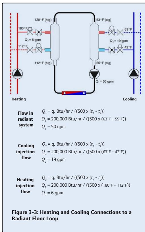
To illustrate this further we will assume the embedded system will have a cooling capacity of 200,000 Btu/hr (63.4 kW).
