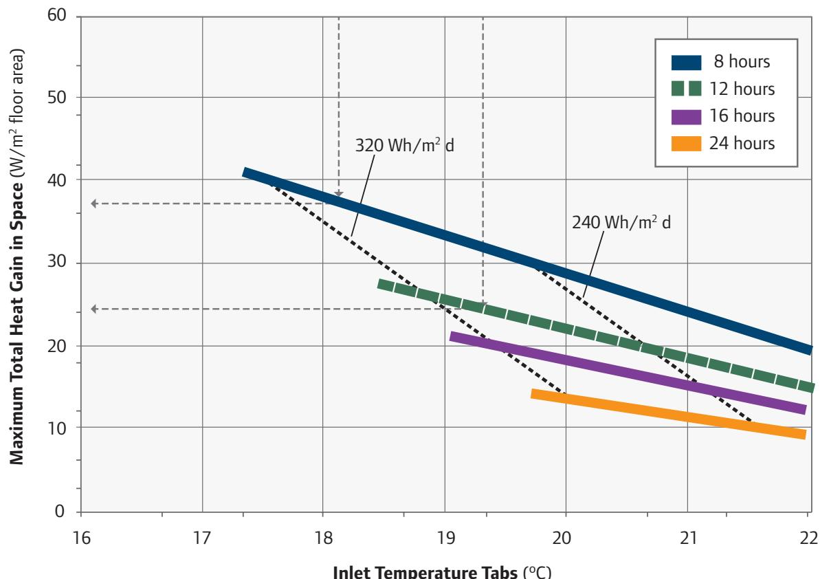
Figure 3-13: Required Cooling Power on the Water Side
