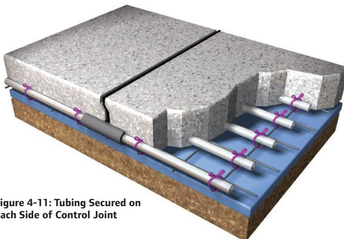
Figure 4-11: Tubing Secured on Each Side of Control Joint
