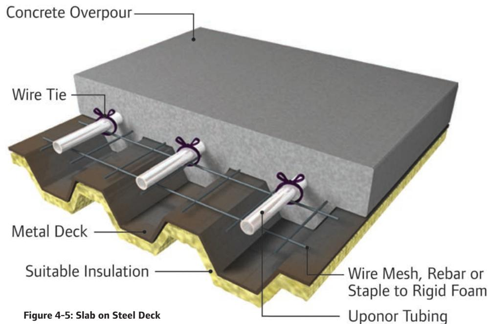
**Figure 4-5: Slab on Steel Deck**
