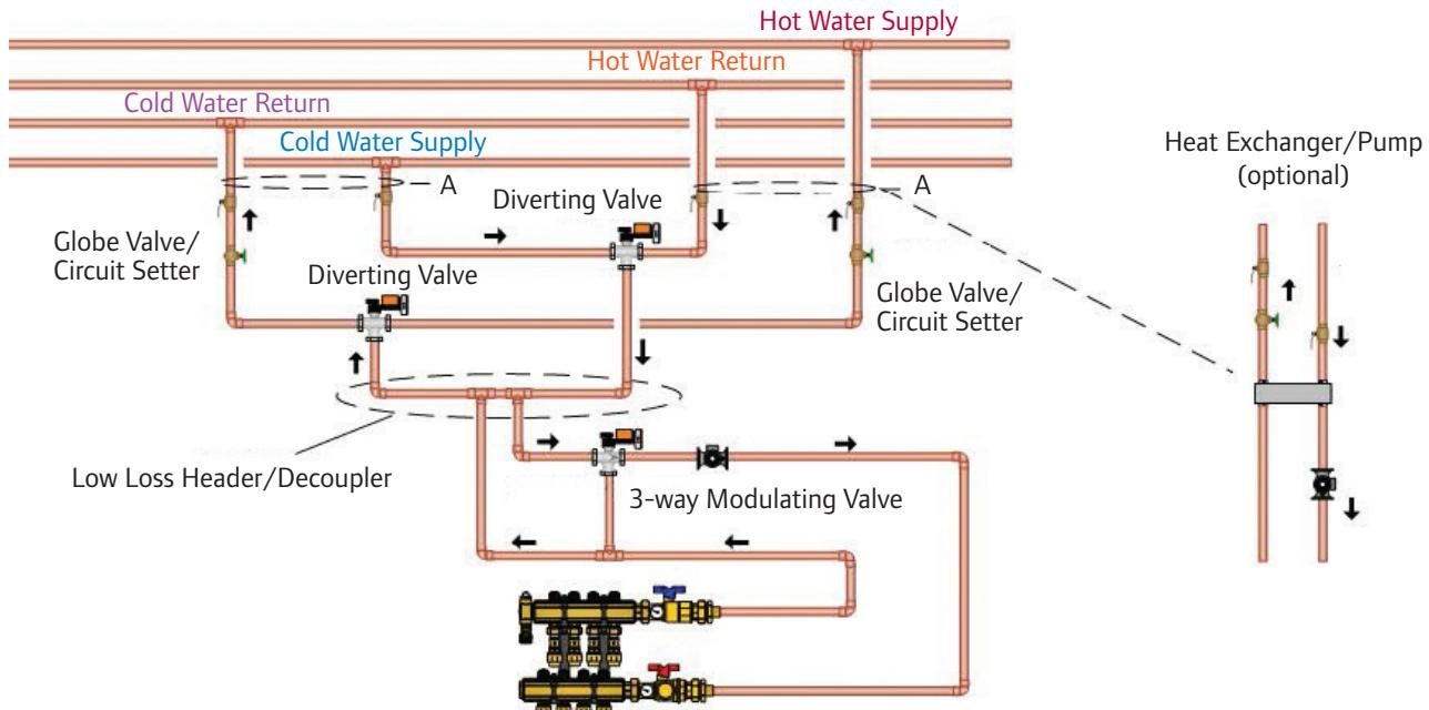
Figure 3-1: Mixing with Heating/Cooling Switchover
