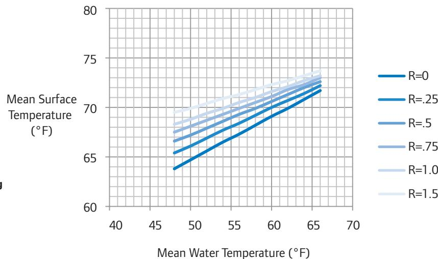
**Figure 4-12: Average Water Temperature Charts for Tubing with 6" O.C. Spacing**
