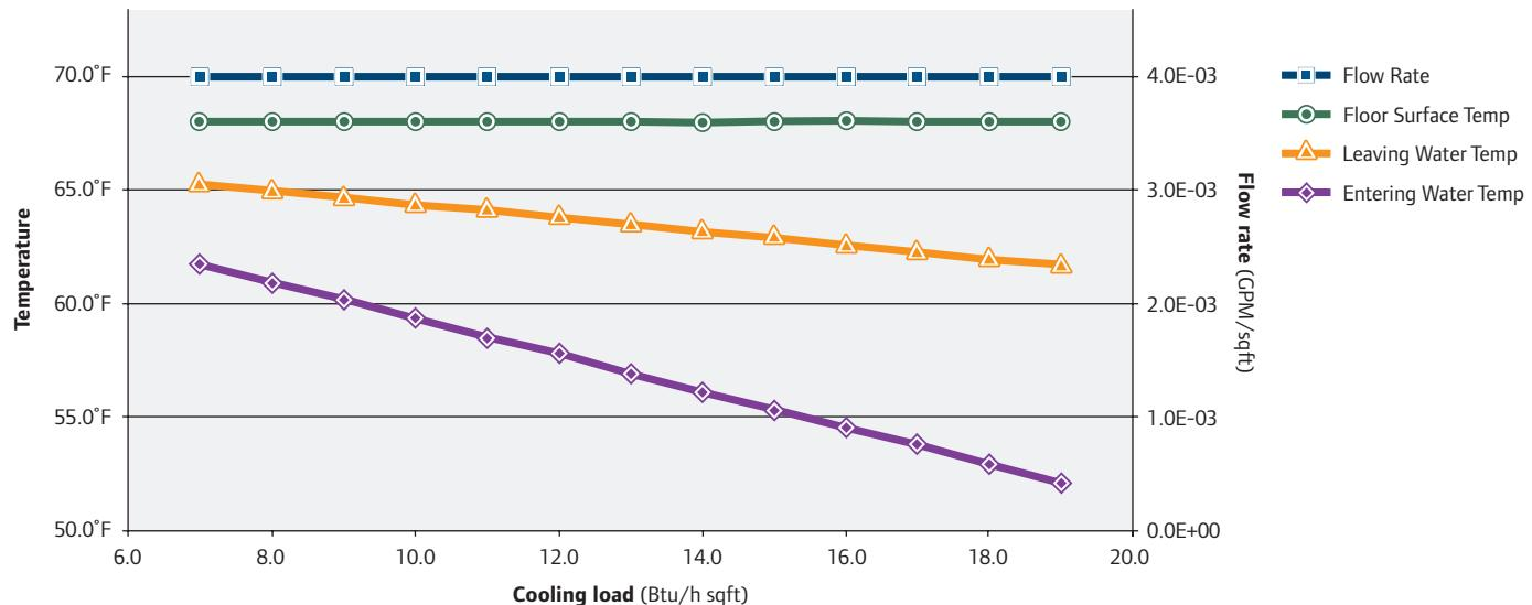
Figure 3-4: Characteristics of a Constant Flow, Variable Temperature Control
