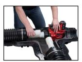
Expand the pipe end. To ensure a uniform expansion, the expander rotates according to the integrated auto rotate function.
