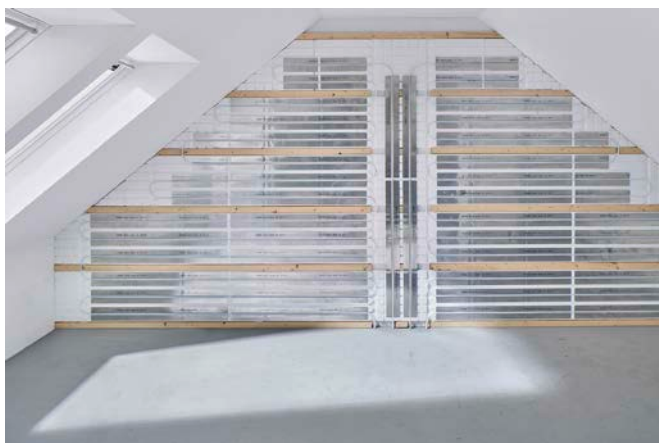
Uponor Siccus plate – laying plate made of EPS with pipe routing channels for holding the Uponor Siccus heat conducting lamellas. Laying spacing 15 / 22.5 / 30 cm.
