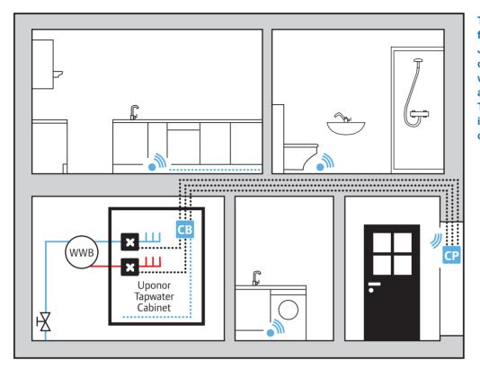
The simplicity and safety for users is significant. Just press the button OFF on the panel in the hallway when leaving the house and ON when returning. This means that the water is always shut off when no one is at home.
