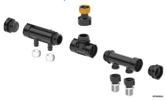
Tee to connect two manifolds - Select manifolds with fixed Q&E outlets or threaded outlets for adapters - Adapter PPM 1" female with  $G^2$ " swivel nut - Uponor S-Press adapter for connecting composite pipes in dimensions 16 or 20 mm - Manifold plug at both ends of the manifold
