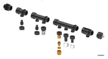
Adapter PPM 1" male with  $G\frac{3}{4}$ " thread - Manifold available with 1, 2, and 3 fixed outlets for various adapters - Manifold end cap with air nipple - Outlet nut to close off unused outlets - Uponor S-Press adapter for connecting composite pipes in dimensions 16 or 20 mm - Uponor FPL-X adapter available in  $G\frac{1}{2}$ " for PE-Xa pipes - Adapters available for Q&E connections to Uponor PE-Xa pipes in both NKB and ISO dimensions 12, 15, 16, 18 and 20 mm
