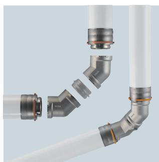
Flexible angles – particularly in old buildings walls and ceilings are often not really at right angles to each other. The short spacers (5 mm) in combination with two 45° elbows allow almost any desired angle to be realised by rotating the components.
