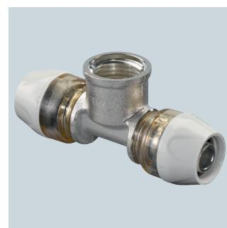
*Uponor RTM tee – with inner thread, – with integrated pressing function, pressed state identification and colour coding, cylindrical inner thread to ISO.*
