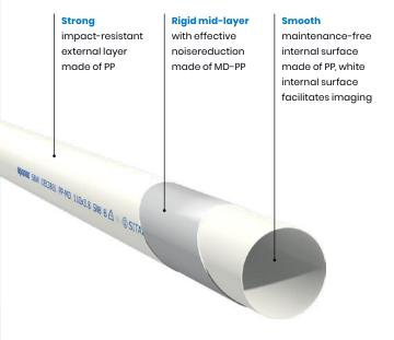
Uponor Decibel is light and easily workable. Compared with a traditional cast iron sewer system, installation can be up to twice as fast. Pipes can be cut off with a saw or pipe cutter, and sleeve couplings make installation quick and easy, even in tight spaces. No hot work is required for installation, so there is no risk of fire. The Decibel angled ground connector is ready to install, making work faster.
