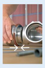
Slide the lock pin into the opening of the fitting body and click it into place
