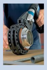
Insert the pressing adapter into the base part.
