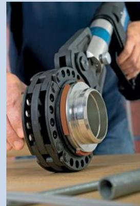
**3** Insert the pressing adapter into the base part.
