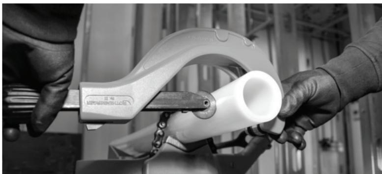
**Figure 13: Swing-style pipe cutter**
