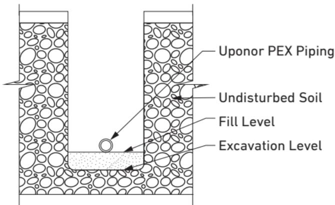
**Figure 10: Poor soil conditions** – With rocky, clay, muddy, or other poor soil conditions, it may be necessary to prepare the trench bottom using granular material of such size and grading to provide a stable base. See local code for additional requirements.
