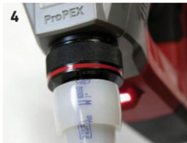
**Figure 28: Expansion with Milwaukee M18 ProPEX Expansion Tool**
