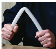
Figure 32: Reforming kinked piping
