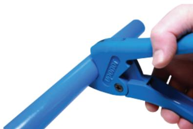
**Figure 15: Square cut pipe with PEX cutter**
