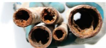
**Figure 7: Corroded metallic pipes**
