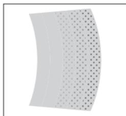
**Figure 4: PEX-c (Radiation) 70-75% crosslinked**
