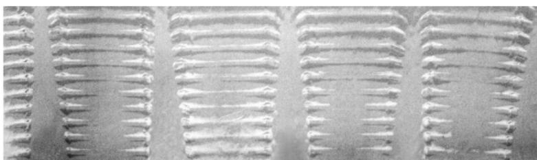
**Figure 30: Expansion without proper rotation**
