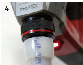
Figure 28: Expansion with Milwaukee M18 ProPEX Expansion Tool
