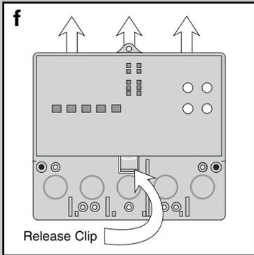
Press the control release clip on the base inside the wiring chamber and slide the control upwards. **(See fig. f)**
