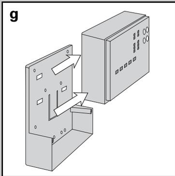
The control lifts up and away from the base. **(See fig. g)**
