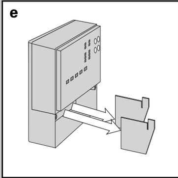
Remove the safety dividers from the wiring chamber by pulling them straight out of their grooves. **(See fig. e)**
