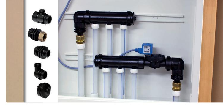
The product range include manifolds with 2,3 and 4 outlets, as well as a single outlet version with either G½" or G¾" male thread. The pitch between the outlets is 50 mm. The single manifold can preferably be used for connecting other parts, such as Q&E Swivel nut 20 or 25 mm, valve solutions and other threaded fittings.
