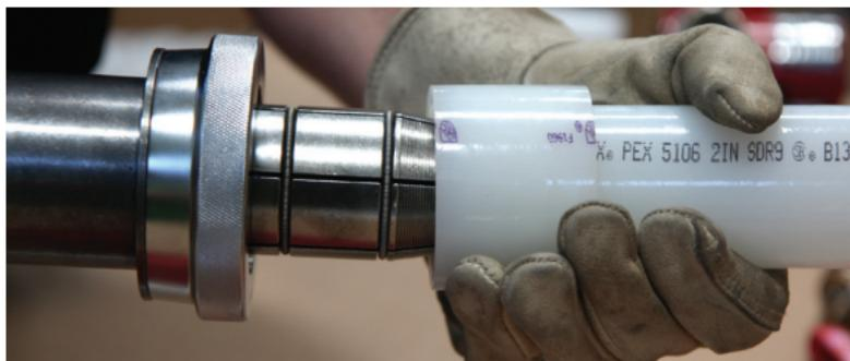
**Figure 22: Slide head into piping**
