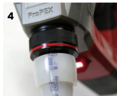
**Figure 9: Expansion with Milwaukee M18 ProPEX Expansion Tool**
