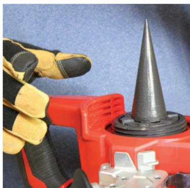
**Figure 10: FORCE LOGIC expansion head installation**
