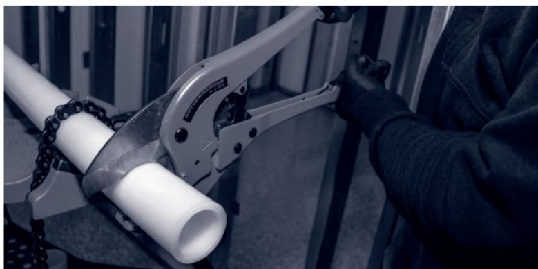
**Figure 34: Uponor ratchet-style pipe cutter for up to 3" pipe (E6083000)**
