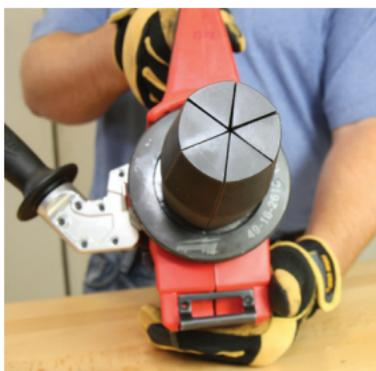
**Figure 13: Correct expansion head alignment**
