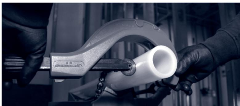
**Figure 33: Uponor swing-style pipe cutter for up to 4" pipe (E6084000)**
